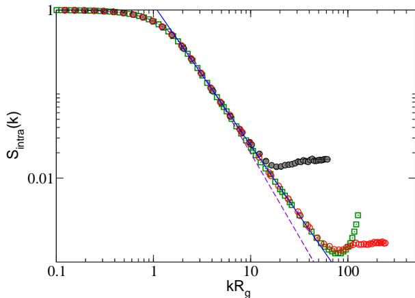
FIG. 2: (Color online) Intramolecular structure factor  $S_{\text{intra}}(k)$  of a single SAW polymer versus  $kR_g$  on a log-log scale. Squares: MC data for an  $L = 1000$  SAW polymer: closed circles and open circles: MC data for  $n = 62$  and  $n = 602$  blob representations. Full line: scaling regime  $1.15(kR_g)^{1/\nu}$ , with  $\nu \simeq 0.5988$ ; dashed line: Debye structure factor for a Gaussian chain.
