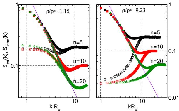
FIG. 3: (Color online) Total (open symbols) and intramolecular (closed symbols) structure factors versus  $kR_g$  from MC simulations of  $n = 5$  (circles),  $n = 10$  (squares) and  $n = 20$  (triangles) blob representations of SAW polymers at  $\rho/\rho^* = 1.15$  (left frame) and  $9.23$  (right frame). The straight lines correspond to the scaling regime as in fig. 2
