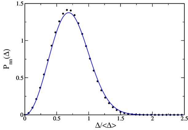
FIG. 5: (Color online) The nearest neighbor spacing distribution  $P_{\text{nn}}(\Delta)$  calculated using the Toeplitz representation Eq. (61) with  $n = 200$  (black points) is in good agreement with the generalized Wigner surmise approximation, Eq. (21) (blue curve).
