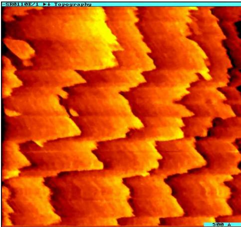
FIG. 1: (Color online) A scanning tunneling microscope image of  $300 \times 300 \text{ nm}^2$  area, showing the surface morphology of a typical SRO film deposited on (100) STO wafer. The observed plates are atomically smooth, and the steps between them are of one unit cell height in the  $c$ -direction of SRO (0.785 nm).
