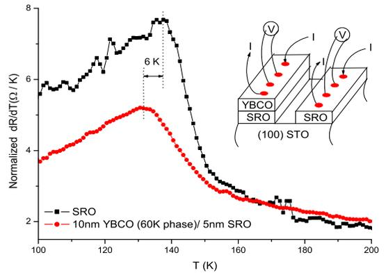
FIG. 7: (Color online)  $dR/dT$  versus temperature of a 10 nm YBCO (60 K phase)/5 nm SRO bilayer normalized to its 5 nm thick SRO reference film on the same wafer. Normalization is done in the 160-180 K temperature range. The inset shows a schematic drawing of the bilayer and reference film on the wafer together with the two four probe contacts configuration.
