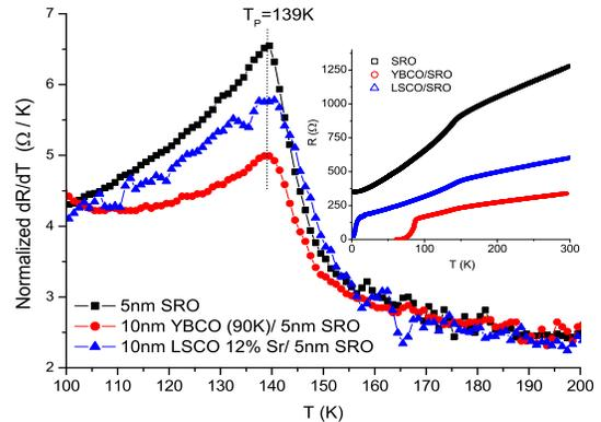
FIG. 8: (Color online) Normalized  $dR/dT$  versus temperature of two bilayers, one of a 10 nm YBCO/5 nm SRO of the 90 K YBCO phase, and the other of a 10 nm  $La_{1.88}Sr_{0.12}CuO_{4-y}$ /5 nm SRO, together with the  $dR/dT$  data of a 5 nm thick SRO reference film. Normalization to the reference film is done in the 160-180 K temperature range. The inset shows the raw data of  $R$  versus  $T$ .
