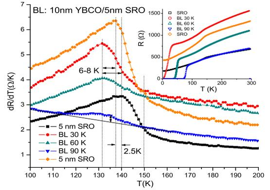
FIG. 6: (Color online)  $dR/dT$  versus temperature of the same 10 nm YBCO/5 nm SRO bilayer reannealed to produce the 30, 60 and 90 K YBCO phases, together with the  $dR/dT$  data of two 5 nm thick SRO films of high and low resistances. The inset shows the corresponding raw data of  $R$  versus  $T$ .
