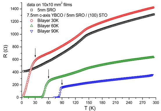
FIG. 3: (Color online) Resistance versus temperature of a 5 nm SRO film, and of a 7.5 nm YBCO/5 nm SRO bilayer reannealed under different conditions to produce YBCO with  $T_c$  of either 90, 60 or 30 K (see the arrows).
