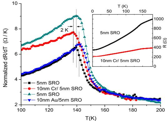
FIG. 9: (Color online)  $dR/dT$  versus temperature of 10 nm Cr/5 nm SRO and 10 nm Au/5 nm SRO bilayers normalized to two 5 nm thick SRO reference films. Normalization is done in the 160-180 K temperature range. The inset shows the raw data of  $R$  versus  $T$  for the Cr bilayer and one of the SRO films.
