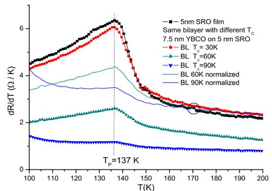
FIG. 4: (Color online) Temperature derivatives  $dR/dT$  of the resistance versus temperature data of Fig. 3. The curves without symbols represent the 60 and 90 K bilayers data normalized to the reference SRO data in the temperature range indicated by the circle.
