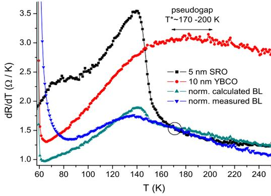
FIG. 5: (Color online) Temperature derivatives  $dR/dT$  of the resistance versus temperature of a 5 nm thick SRO film and a 10 nm thick 60 K YBCO film together with the normalized data of the measured and calculated results of 10 nm YBCO/5 nm SRO bilayers. The bilayer curves are normalized to the reference SRO data at 170 K as indicated by the circle.
