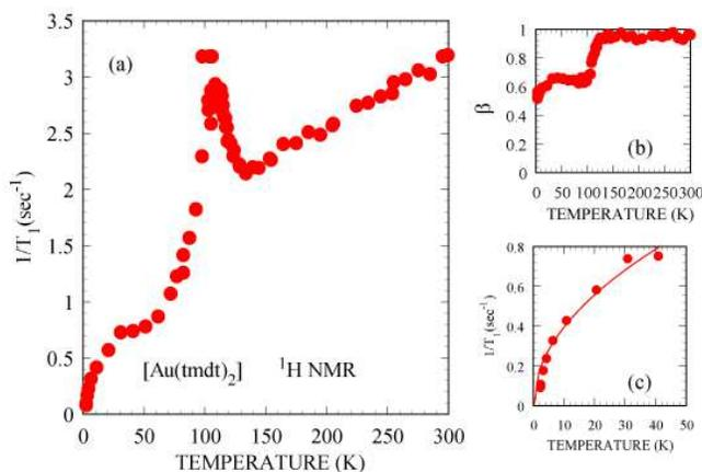
Fig. 6. (Color online) (a) Temperature dependence of  $1/T_1$ . Above 110 K,  $1/T_1$  is unambiguously determined from a simple exponential recovery curve of nuclear magnetization. Below 110 K,  $1/T_1$  is determined by a stretched exponential function,  $\exp[-(t/T_1)^\beta]$ , fitting the non-single exponential recovery. (b) Temperature dependence of fitting parameter  $\beta$ . (c) Temperature dependence of  $1/T_1$  at low temperatures. The solid line expresses  $T^{0.5}$ .
