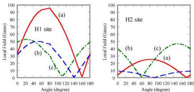
Fig. 5. (Color online) Parallel component of the local field. (a), (b), and (c) correspond to the spin structures shown in Fig.4. The external field is parallel to the longest direction of the molecule. The moment is rotated within the plane perpendicular to the external field.
