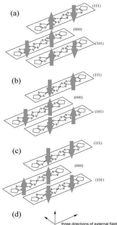
Fig. 4. Spin structures assumed in the calculations. Pattern (a) is suggested by the first principle band calculation.<sup>13</sup> (d) shows the directions of the external field assumed in the calculations
