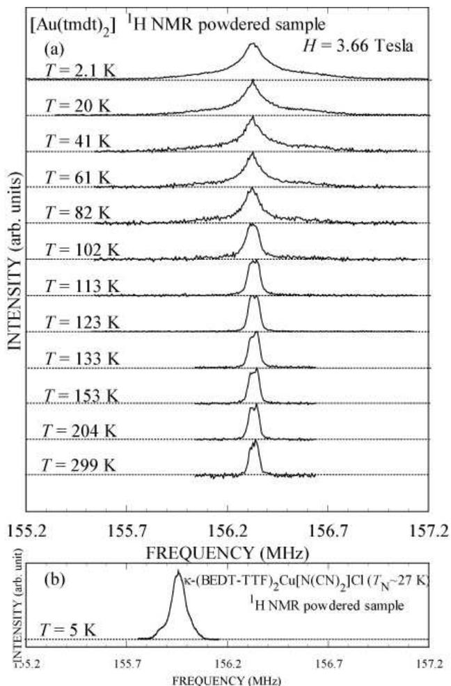
Fig. 2. (a)  $^1\text{H}$  NMR spectra of powdered  $[\text{Au}(\text{tmdt})_2]$ . (b)  $^1\text{H}$  NMR spectrum of powdered  $\kappa\text{-(BEDT-TTF)}_2\text{Cu}[\text{N}(\text{CN})_2]\text{Cl}$  at 5 K well below  $T_N$ . The difference between the spectral centers of the two salts is due to the difference in their fields.
