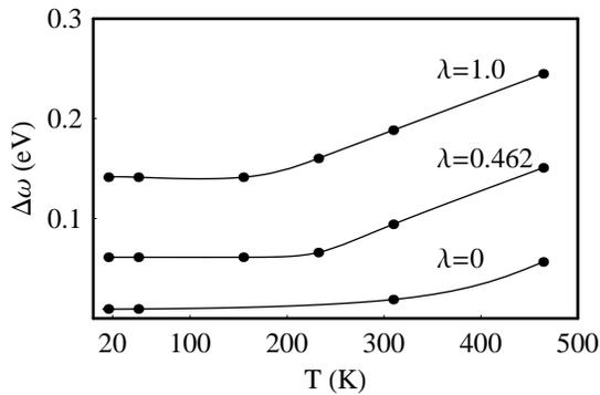
FIG. 4: The peak's width,  $\Delta\omega$ , as a function of the temperature,  $T$ , for the t-J model ( $\lambda = 0$ ) and in strong EPI limit ( $\lambda = 0.462$  and  $\lambda = 1$ ). The temperature  $T$  is defined in units of Kelvin assuming  $t = 0.4\text{eV}$ .
