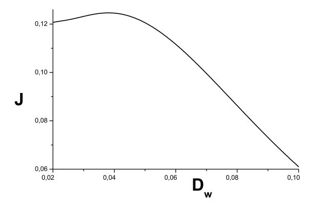
FIG. 3: Net current J for a gaussian white noise, as function of  $D_w$ . The values of parameters are A = 1, l = 1,  $U_r = 0.16$  and  $U_b = 0.2512$ .
