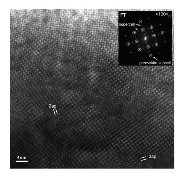
**FIG. 1.** HREM image corresponding to one of the perovskite  $\{100\}$  planes showing the nanostructurally ordered LaBaCo<sub>2</sub>O<sub>6</sub> has 90° oriented domains in the 112-type ordered phase. The inset figure shows Fourier transform (FT) of the main figure and the strong reflections related to the perovskite subcell. Two supplementary sets of reflections are observed and related to the existence of 90° oriented domains having the  $a_p \times 2a_p$  112-type ordered structure.
