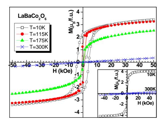
**FIG. 3.** (Color online) Field variation of magnetization (M-H) for LaBaCo<sub>2</sub>O<sub>6</sub> at four different temperatures. The inset figure shows typical hysteresis curves at two different temperatures for completely disorder La<sub>0.5</sub>Ba<sub>0.5</sub>CoO<sub>3</sub> phase.
