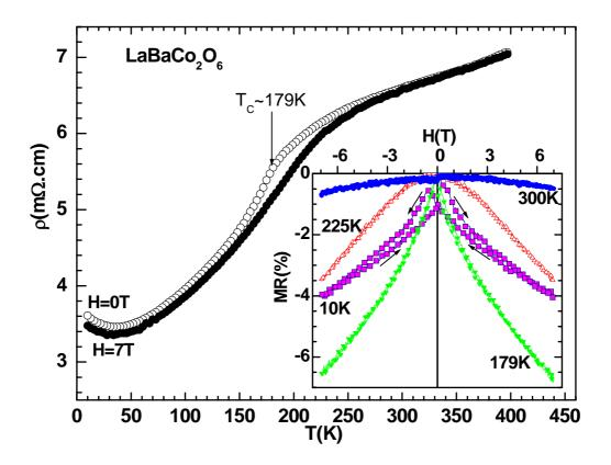
**FIG. 5.** (Color online) Temperature dependence of electrical resistivity,  $\rho$ , of LaBaCo<sub>2</sub>O<sub>6</sub> in the presence (solid symbol) and absence (open symbol) of magnetic field (7 Tesla). The inset figure shows magnetoresistance, MR, at four different temperatures.
