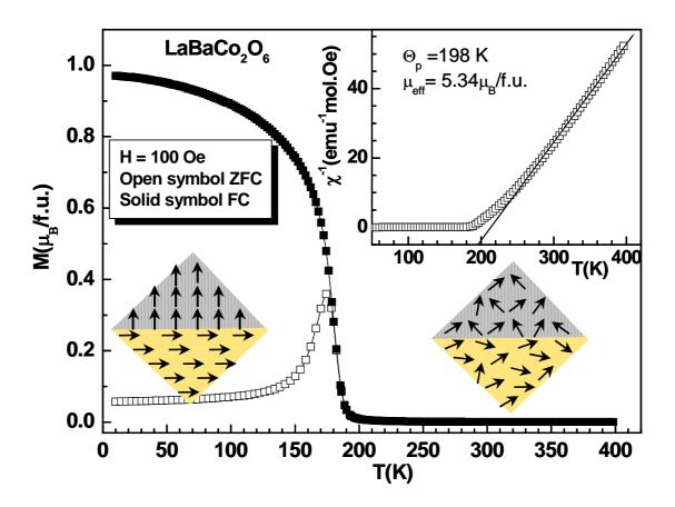
**FIG. 2.** Temperature dependence ZFC (open symbol) and FC (solid symbol) magnetization, M, of LaBaCo<sub>2</sub>O<sub>6</sub> (H = 100 Oe) and the schematic diagrams show the existence of magnetic spins in the 90° oriented nano-domains during ZFC (below and above  $T_C$ ). The inset figure shows inverse susceptibility,  $\chi^{-1}$ , vs temperature plot.
