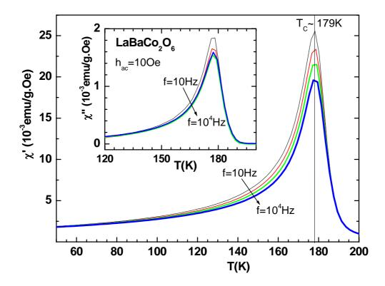
**FIG. 4.** (Color online) The temperature dependence in-phase component of acsusceptibility,  $\chi'$ , of LaBaCo<sub>2</sub>O<sub>6</sub> at four different frequencies (h<sub>ac</sub> = 10 Oe) and corresponding out-of-phase component,  $\chi''(T)$ , data is shown in inset figure.
