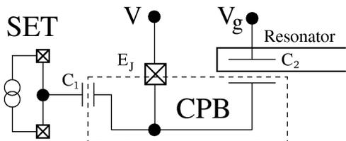
FIG. 1: The circuit diagram for the QND measurement scheme:  $V$  and  $V_g$  are applied voltages, and  $C_1$  and  $C_2$  are the capacitances connecting the three mesoscopic elements. The Cooper-pair box (indicated with a dashed box) is coupled to the nano-resonator and the single-electron transistor.
