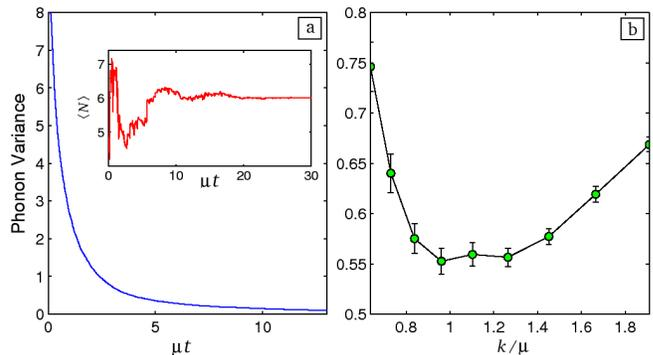
FIG. 2: (a) The evolution of the phonon-number variance of the resonator for  $k = \mu$  averaged over a thousand measurements. Inset: The average value of the phonon number for a single measurement. (c) This average variance as a function of  $k$  after measuring for a time  $t = 2\pi/\mu$ .
