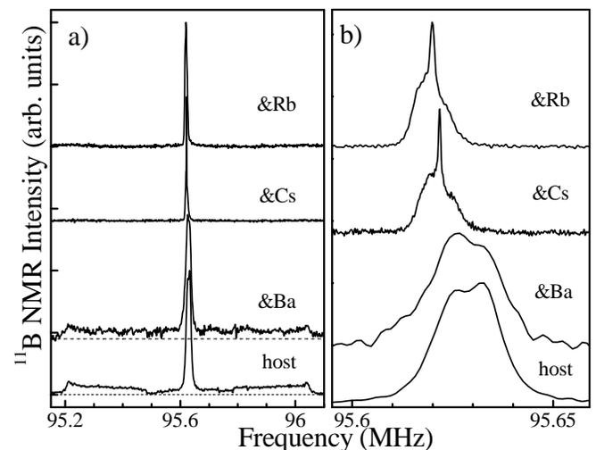
FIG. 2: Room-temperature  $^{11}\text{B}$  NMR spectra at 7 T in the host  $\text{MgB}_2/\text{Mg}$  and in  $\text{MgB}_2/\text{Mg}$  reacted with Ba, Cs, and Rb: The spectra in whole (a) and details of the central peaks (b).
