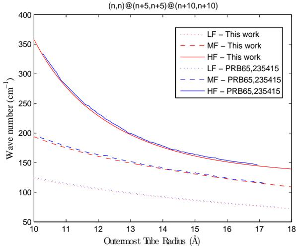
Furthermore, we show the dependence of the RBLM frequencies on the number of layers in Fig. 3, in which the radius of the innermost tube is fixed at  $30 \text{ \AA}$ . This result matches the Fig. 6 of Ref. 12 perfectly. Based upon Fig. 3, a new method to determine the number of layers for the MWCNTs can be proposed, i.e., if the position of the lowest RBLM for a MWNT is obtained, one can easily find out how many layers are present in the MWCNT by comparing the experimental data with Fig. 3.
