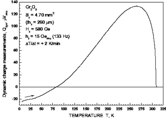
FIG. 8: Magnetolectric susceptibility  $\alpha_{||}(T)$  for  $\text{Cr}_2\text{O}_3$  obtained by low frequency (133 Hz) AC  $\text{ME}_H$  experiments ( $h_z \approx 18 Oe_{\text{rms}}$ ). Knowing  $T \approx 85.0 K$  at  $\alpha_{||}(T) = 0$  from quasi-static experiments and the base line above  $T_N$ , the curve was corrected for a small drift.
