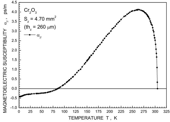
FIG. 6: Magnetolectric susceptibility  $\alpha_{||}(T)$  for  $\text{Cr}_2\text{O}_3$ , obtained by quasi-static  $\text{ME}_H$  experiments,  $H$  varying at each temperature from 0 to 10 kOe and back to 0, as described in the text. The interpolation between the points was made by means of B-splines and is only a guide for the eyes.
