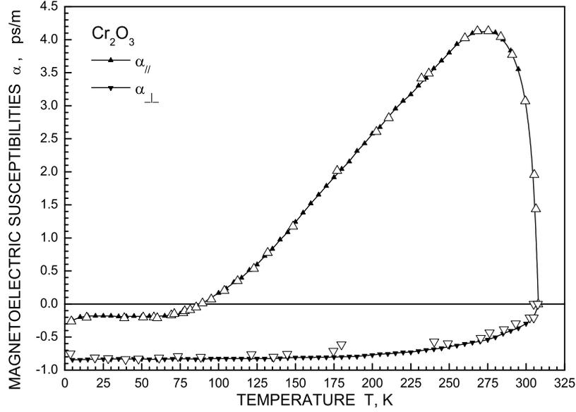
FIG. 2: The  $ME_H$  effect (linear magnetoelectric effect with magnetic field-induced polarization) of  $Cr_2O_3$ : Plot of  $\alpha_{||}(T)$  and  $\alpha_{\perp}(T)$  after digitalization and interpolation (small full triangles) of Fig.2.8, p.41, of Wiegmann [88], (see also Fig.2, p.143, Wiegmann et al. [90]). The sign of  $\alpha_{\perp}(T)$  was set negative according to Astrov [3]. The curves (B-Splines) are only guides for the eyes.
