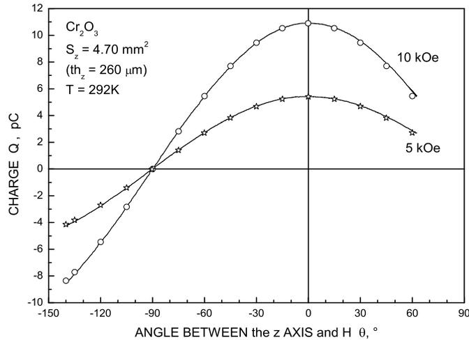
FIG. 7:  $\text{ME}_H$  experiments for  $\text{Cr}_2\text{O}_3$  at  $T = 292 \text{ K}$  and constant  $H$  fields. By rotating the electromagnet, the measured charges (continuous lines) follow cosine curves. Superimposed are normalized computed points (open circles at  $H = 10 \text{ kOe}$ , open stars at  $H = 5 \text{ kOe}$ ). This proves that  $\alpha_{zx}$  and  $\alpha_{zy}$  are very small or null. At  $\theta = 0^\circ$ , the field  $H$  is parallel to the optical axis ( $z$  axis).
