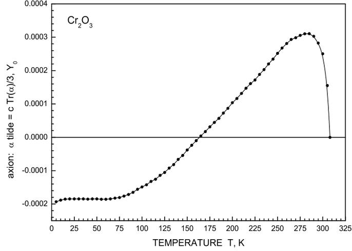
FIG. 9: The pseudoscalar or axion piece  $\tilde{\alpha}$ , see Eq.(4), of the constitutive tensor  $\chi^{\lambda\nu\sigma\kappa}$  of  $\text{Cr}_2\text{O}_3$  in units of  $Y_0 = 1/Z_0$  as a function of the temperature  $T$  in *kelvin*; here  $Z_0$  is the vacuum impedance which, in SI, is  $\approx 377 \text{ ohm}$ .
