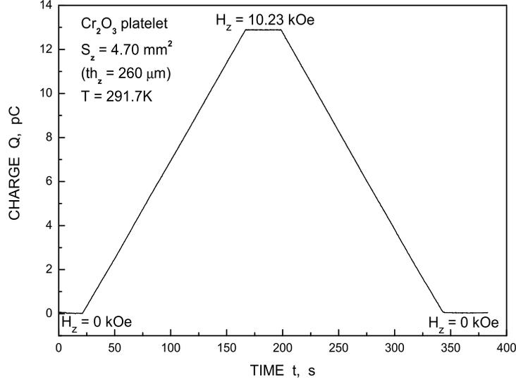
FIG. 5: Quasi-static  $ME_H$  experiment for  $Cr_2O_3$ , charge vs. time. The field  $H$  varies linearly in time, from 0 to 10 kOe and from 10 kOe to 0, proving the linearity of the magnetoelectric effect in  $Cr_2O_3$ , here for  $\alpha_{||}$  (at 292 K).
