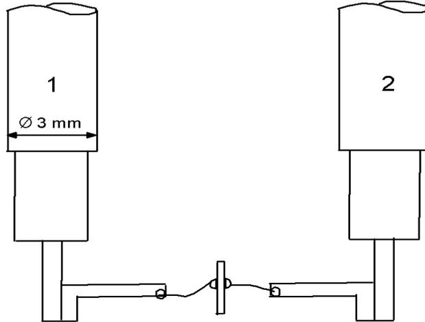
FIG. 4: a) A  $\text{Cr}_2\text{O}_3$  platelet ( $S_z = 4.70 \text{ mm}^2$ ,  $th_z = 260 \mu\text{m}$ ) for  $\alpha_{||}(T)$  measurements, connected to two low noise coaxial cables #1 and #2. One can see, by reflection on the platelet, the gold wire and the Cu wire #2 to the right. Black lines were added on the right of this unique Polaroid picture for clarity. b) A schematic drawing of the set-up depicted under a).
