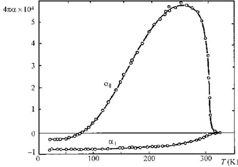
FIG. 1: The  $\text{ME}_E$  effect (linear magnetolectric effect with electric field-induced magnetization) of  $\text{Cr}_2\text{O}_3$ : Temperature dependence of the magnetolectric components  $\alpha_{\parallel}$  and  $\alpha_{\perp}$  according to Astrov [3], see also the Tables [5].
