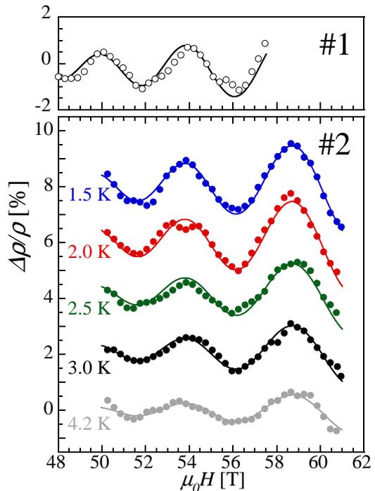
FIG. 2: (Color online). The oscillatory component of the magnetoresistance  $[\Delta\rho/\rho(H)]$  for both samples at various temperatures. For #1,  $\rho = \rho_{xx}(H)$  whilst for #2,  $\rho$  is a mixture of  $\rho_{yy}(H)$  and  $\rho_{xy}^H(H)$ . In each case, a linear background has been subtracted and the data offset for clarity. The solid lines are fits to Eq. (1) giving  $m^* = 2.7 \pm 0.3m_e$ .
