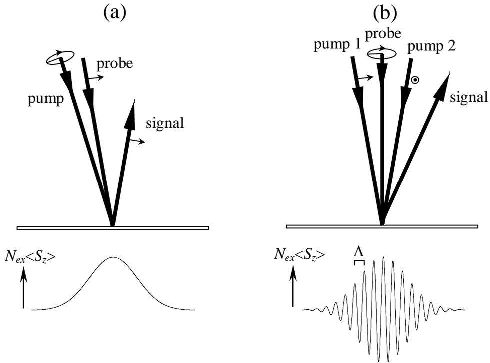
**Figure 1.** Experimental configurations for measurements of (a) spin relaxation and (b) spin diffusion. Upper diagrams, incident pump and probe beams and their polarisations; lower diagrams, profile of focussed pump spot with (a) a spin polarised population and (b) spin grating with spacing  $\Lambda$ .
