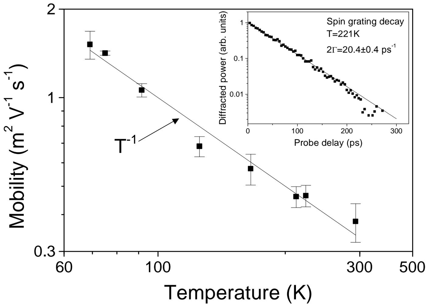
**Figure 3.** Logarithmic plot of the electron mobility, in a sample from the same wafer as data of Fig.2, determined by the spin-grating method. The electric field is the built-in field of the *pin* structure,  $2.80 \cdot 10^6 \text{ Vm}^{-1}$ . The  $T^{-1}$  temperature dependence is as expected for a non-degenerate two-dimensional electron system with dominant phonon scattering. Inset is a typical grating decay signal at 221 K.
