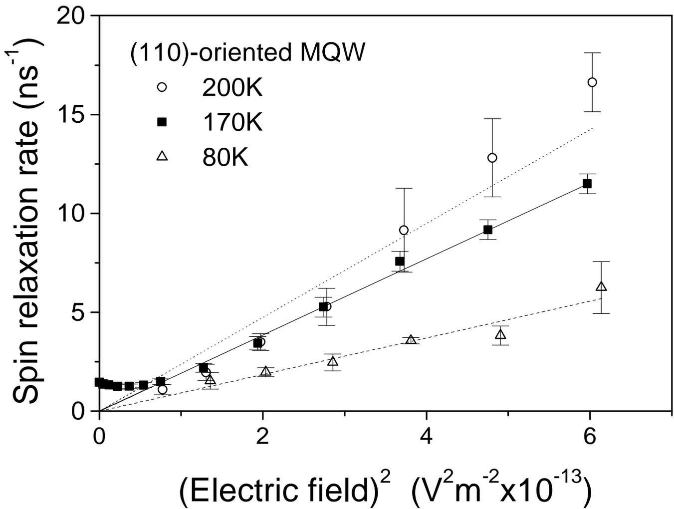
**Figure 2.** Electric field dependence of spin relaxation rate at three temperatures. The high field linear regions of the graphs extrapolate to the origin and the slopes are used to determine the Rashba coefficient
