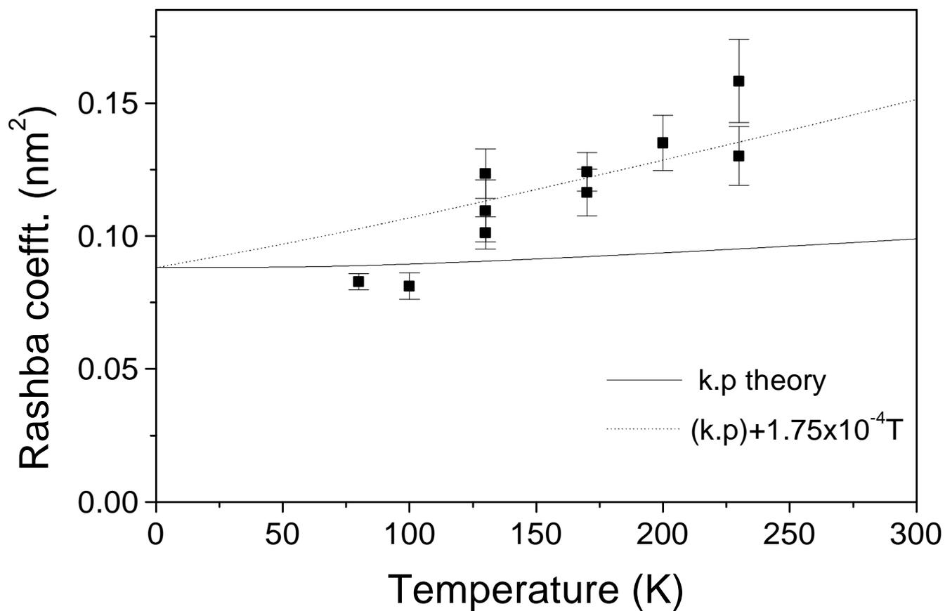
**Figure 4.** Rashba coefficient obtained from combination of spin relaxation and mobility measurements. Solid curve is 8-band **k.p** calculation including temperature dependence of band edges and of interband momentum matrix element. Dotted curve is k.p theory plus an empirical linear-in- $T$  term.
