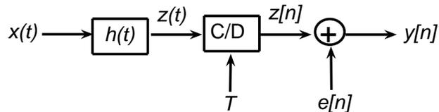
Fig. 1. Block diagram showing our problem setup.  $x(t)$  is a signal with FRI given by (1) and  $h(t)$  is the Gaussian filter with width  $\sigma_h$  given by (2).  $e[n]$  is i.i.d. Gaussian noise with standard deviation  $\sigma_e$  and  $y[n]$  are the noisy samples. From  $y[n]$  we will estimate the parameters that describe  $x(t)$ , namely  $\{c_k, t_k\}_{k=1}^K$ , and  $\sigma_e$ , the standard deviation of the noise.
