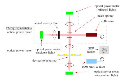
Fig. 2. Schematic of the optical setup used to measure the optical absorptance. A state of polarization (SOP) locker was used to set the input polarization of the incident 1.55- $\mu$ m-wavelength light. Light was focused to a 4  $\mu$ m (FWHM) spot onto a device and the incident, reflected, and transmitted power were measured. The absorptance was calculated from these measurements and earlier calibrations discussed in the main text.
