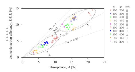
Fig. 5. Plot of device detection efficiency as a function of absorptance for the same devices. Dotted lines have a constant slope given by  $P_{\rm R}$ , the probability of resistive state formation.
