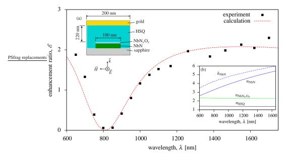
Fig. 6. Plot of enhancement factor,  $\mathscr{E}$  as a function of wavelength  $\lambda$ . The dotted line shows the calculation that was carried out on the unit cell shown in inset (a) using values for the refractive indices shown in inset (b).
