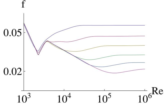
FIG. 1: Analytic reconstruction of Nikuradse’s data, as given in [7], extrapolated to the range up to  $\mathbf{Re} = 10^6$ , actually covered in the Princeton Super Pipe experiment. The six lines correspond, from the bottom up, to  $\epsilon^{-1} = 507, 252, 126, 60, 30.6$  and  $15$ . Both scales are logarithmic.
