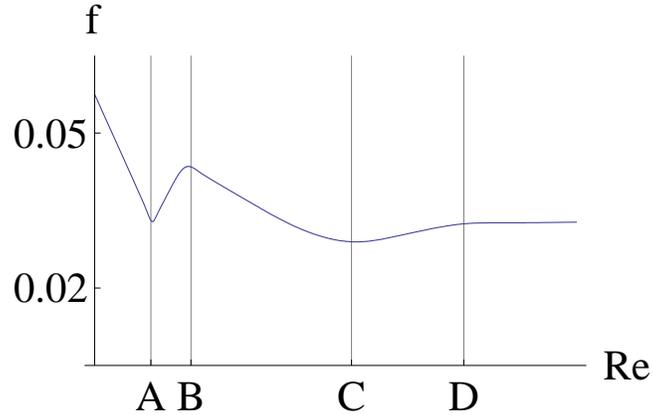
FIG. 2: A close up of the curve corresponding to  $\epsilon^{-1} = 126$ . Observe the sharp minimum at  $A$ , the hump at  $B$  and the belly at  $C$ . To the right of  $D$  the friction factor is constant.
