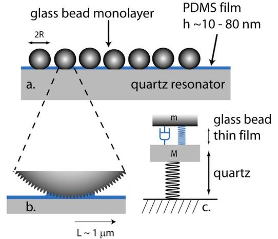
FIG. 1: Sketch of the experiment and modeling of the system
