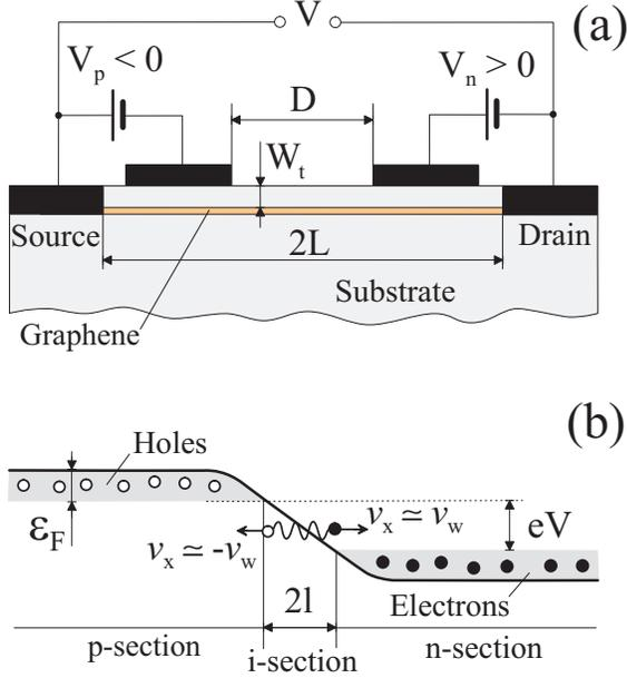
FIG. 1: Schematic view of a G-TUNNETT structure (a) and its band diagram (b).
