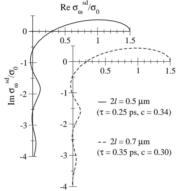
FIG. 3: Real part vs imaginary part dependence with  $\omega\tau$  as a parameter for different length of i-section (different transit times and normalized capacitances).
