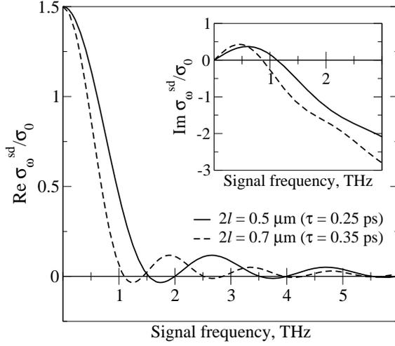
FIG. 2: Real part and imaginary part (inset) of the ac conductance  $\sigma_{\omega}^{sd}$  as functions of signal frequency  $f = \omega/2\pi$  for different lengths of i-section (different transit times).
