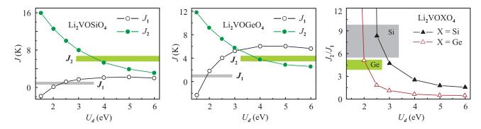
FIG. 5: (Color online) Exchange couplings in  $\text{Li}_2\text{VOSiO}_4$  (left panel) and  $\text{Li}_2\text{VOGeO}_4$  (middle panel) calculated for different values of Coulomb repulsion parameter  $U_d$  and the resulting frustration ratios  $J_2/J_1$  for both the compounds (right panel). Shaded stripes show experimental estimates from Refs. 18,19,20 and 25.
