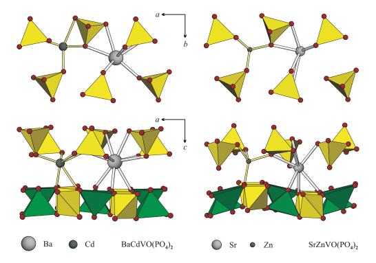
FIG. 6: (Color online) Crystal structures of  $BaCdVO(PO_4)_2$  (left panels) and  $SrZnVO(PO_4)_2$  (right panels): the upper panels show the interlayer  $[AA'PO_4]$  blocks, while the bottom panels present the buckling of the  $[VOPO_4]$  layers. The change of Ba and Cd for Sr and Zn leads to the reduction of the coordination numbers and the resulting reorganization of the structure: the layer buckling and the stretching in the ab plane (see text for details).
