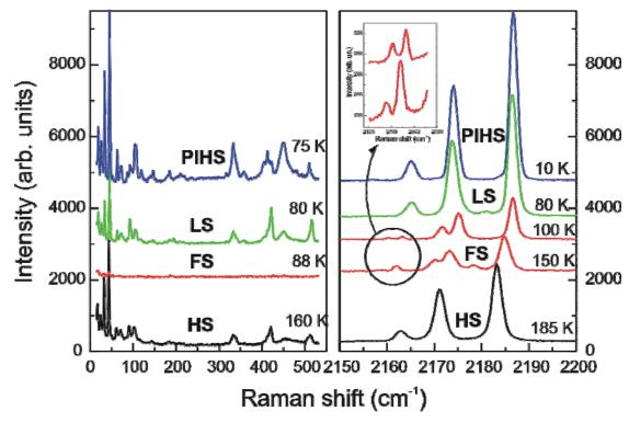
Fig. 3. Temperature dependent Raman spectra of the  $[Fe(pmd)(H_2O)\{Au(CN)_2\}_2]\cdot H_2O$  measured in the frequency regime of  $0-550~\text{cm}^{-1}$  and  $2150-2200~\text{cm}^{-1}$ . The inset shows details of the spectra in the FS state phase.
