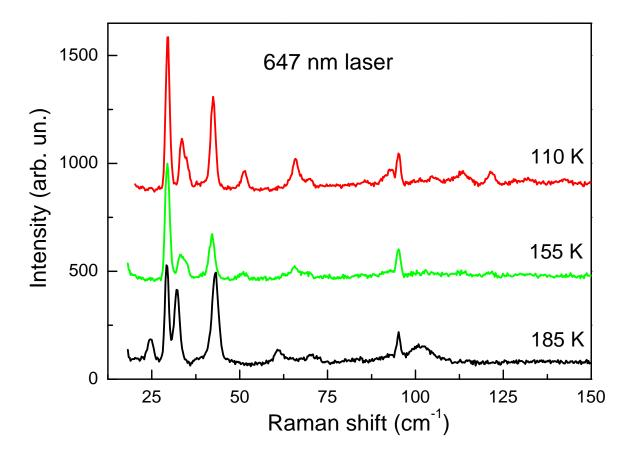
Fig. 7. Raman spectra of the  $[Fe(pmd)(H_2O)\{Au(CN)_2\}_2] \cdot H_2O$  excited by a red-647 nm laser line.
