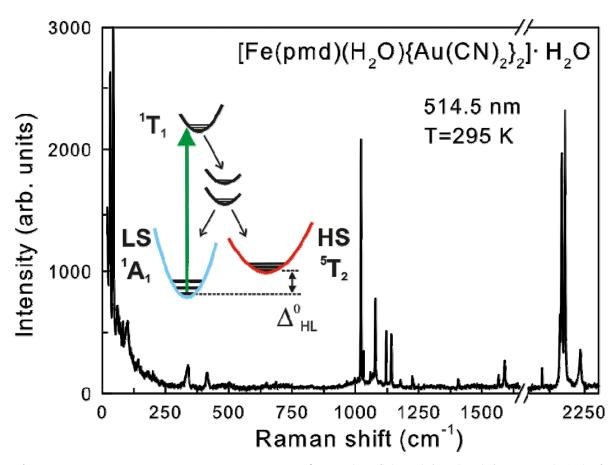
Fig. 2. Room-temperature Raman spectrum of a  $[Fe(pmd)(H_2O)\{Au(CN)_2\}_2]\cdot H_2O$  (**1Au**) single crystal. The inset shows a sketch of the spin state diagram including a light induced excitation with a 514nm laser line.
