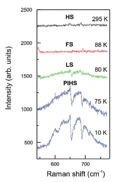
Fig. 8. Fano resonance in the PIHS phase of  $[Fe(pmd)(H_2O)\{Au(CN)_2\}_2]\cdot H_2O$ .
