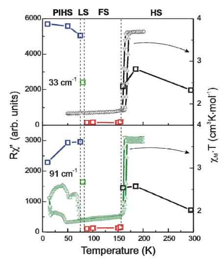
Fig. 5. Temperature dependence of integrated Raman intensities  $R\chi$ " for selected low frequency phonon lines (33 and 91 cm<sup>-1</sup>, open squares in upper and lower plot, respectively) and the susceptibility  $\chi_M T$  without light irradiation <sup>23</sup> (triangles, upper right scale) and under laser ( $\lambda = 540$  nm) irradiation (triangles, lower right scale).
