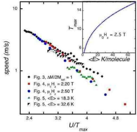
FIG. 7: Avalanche speed vs. the ratio  $U/T_{max}$ , where  $U$  is the calculated barrier and  $T_{max}$  is the maximum flame temperature. The inset shows  $T_{max}$  calculated from the heat capacity at  $2.5\text{ T}$  as a function of  $\langle E \rangle$ .
