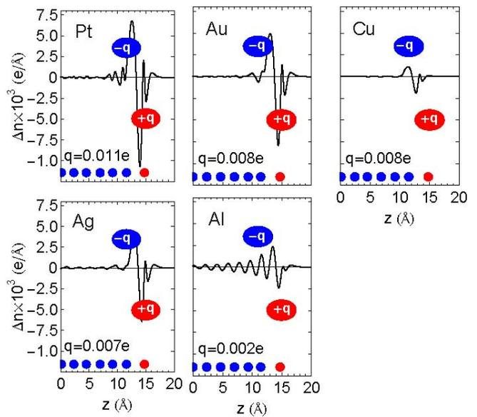
FIG. 5: (Color online) Plane-averaged electron difference density  $\Delta n(z)$  (per unit cell) showing the charge displacement upon physisorption of graphene on M(111) surfaces where M = Al, Ag, Cu, Au, and Pt.  $q/e$  is the number of electrons per carbon atom calculated by integrating  $\Delta n(z)$  from the central node to infinity.<sup>61</sup>
