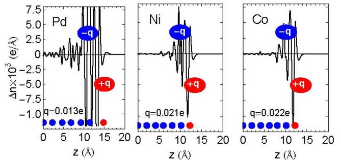
FIG. 7: (Color online) Plane-averaged electron difference density  $\Delta n(z)$  (per unit cell) showing the charge displacement upon formation of the chemisorbed graphene-M(111) interface, with M = Ni, Co, Pd.  $q$  is the charge (per carbon atom) calculated by integrating  $\Delta n(z)$  from the central nodal point to infinity.<sup>61</sup>
