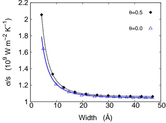
FIG. 5: Thermal conductance in  $\theta = 0$  and  $\pi/2$  directions versus width of graphene strip. Lines are guide to the eye.
