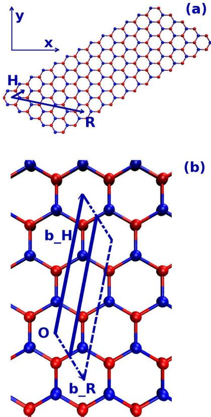
FIG. 1: Graphene strip is described by a lattice vector  $\vec{R} = n_1\vec{a}_1 + n_2\vec{a}_2$ . (a). Strip with  $(n_1, n_2) = (4, 2)$  and  $(N_H, N_R) = (12, 1)$ ; (b). The Brillouin zone for this special strip is two discrete segments (solid) in the reciprocal space.
