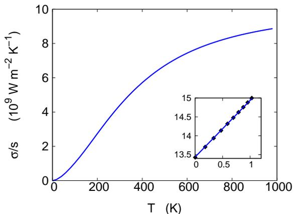
FIG. 3: The thermal conductance of the graphene sheet v.s. temperature. Inset is  $\log \tilde{\sigma}$  v.s.  $\log T$  in extremely low temperature region. The calculated results (filled squares) can be fitted by function  $f(x) = 13.44 + 1.5x$  (blue line). It indicates that the thermal conductance has a  $T^{1.5}$  dependence in this region.
