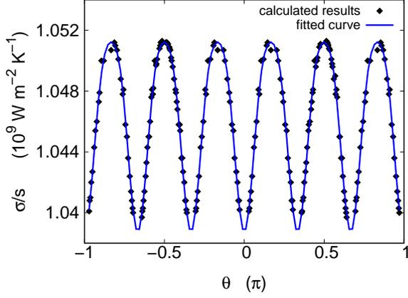
FIG. 4: The direction dependence of thermal conductance.  $\theta$  is the direction angle for the thermal flux. The calculated results (filled squares) are fitted by the function  $f(x) = a + b \cos(6\theta) + c \cos(12\theta)$  with  $a = 1.0456 \times 10^9$ ,  $b = -6.237 \times 10^6$  and  $c = -9.642 \times 10^5$ .
