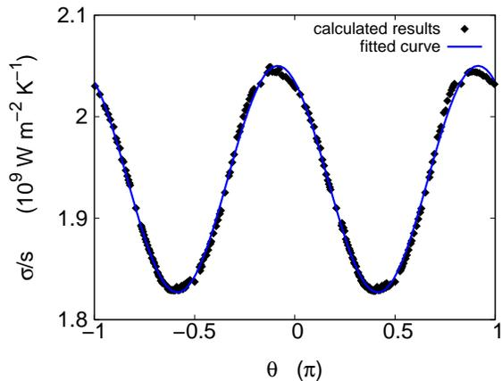
FIG. 11: (Color online) The directional dependence for the thermal conductance of dimerite. The calculated results (filled squares) are fitted by function  $f(x) = a + b \cos(2(\theta + c))$  with  $a = 1.9 \times 10^9$ ,  $b = 1.1 \times 10^8$ , and  $c = 0.1\pi$  (blue line).
