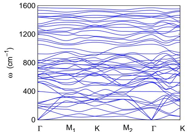
FIG. 9: (Color online) Phonon spectrum for the dimerite along high symmetry lines in the Brillouin zone. Around  $\Gamma$  point, there are low frequency optical modes with frequency about  $200$   $\text{cm}^{-1}$ , which do not exist in pure graphene.
