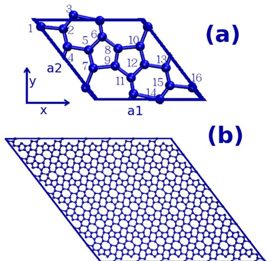
FIG. 8: (Color online) Configuration for the dimerite. (a) is one unit cell for dimerite. There are 16 atoms in each unit cell. The length for the two unit vectors are 7.60 Å and 7.05 Å. The angle between them is  $0.7\pi$ . (b) shows 49 unit cells together.
