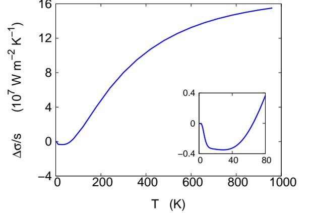
FIG. 7: The difference of the thermal conductance between directions of  $\theta = 0$  and  $\pi/2$  versus temperature. This quantity has an abundant temperature dependence. Inset is the enlarged figure for the low temperature region.
