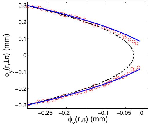
Figure 2: (Color online) The measured crack tip profile ( $\phi_y(r, \pm\pi)$  vs.  $\phi_x(r, \pi)$ ) at  $v=0.2c_s$  (circles). Shown are the parabolic LEFM best fit (dashed line) and the profile predicted by the weakly nonlinear solution (solid line) with  $K_I = 1070\text{Pa}\sqrt{m}$  and  $T = -2800\text{Pa}$ . The values of  $K_I$  used here and in Fig. 1 differ by a few percent, which is consistent with the omission of a correction of order  $T/\mu$  mentioned below Eq. (12).
