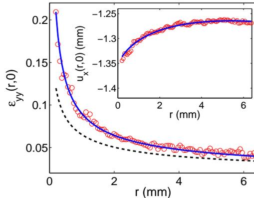
Figure 1: (Color online) Inset: The measured  $u_x(r, 0)$  at  $v = 0.2c_s$  (circles) fitted to the weakly nonlinear solution (solid line) with  $K_I = 1040\text{Pa}\sqrt{m}$  and  $T = -2800\text{Pa}$ . Main panel: The corresponding measurements of  $\varepsilon_{yy}(r, 0) = \partial_y u_y(r, 0)$  (circles) compared to the weakly nonlinear solution (solid line) using the same  $K_I$  and  $T$ . The LEFM prediction (analysis as in Livne et al. (2008)) is added for comparison (dashed line).
