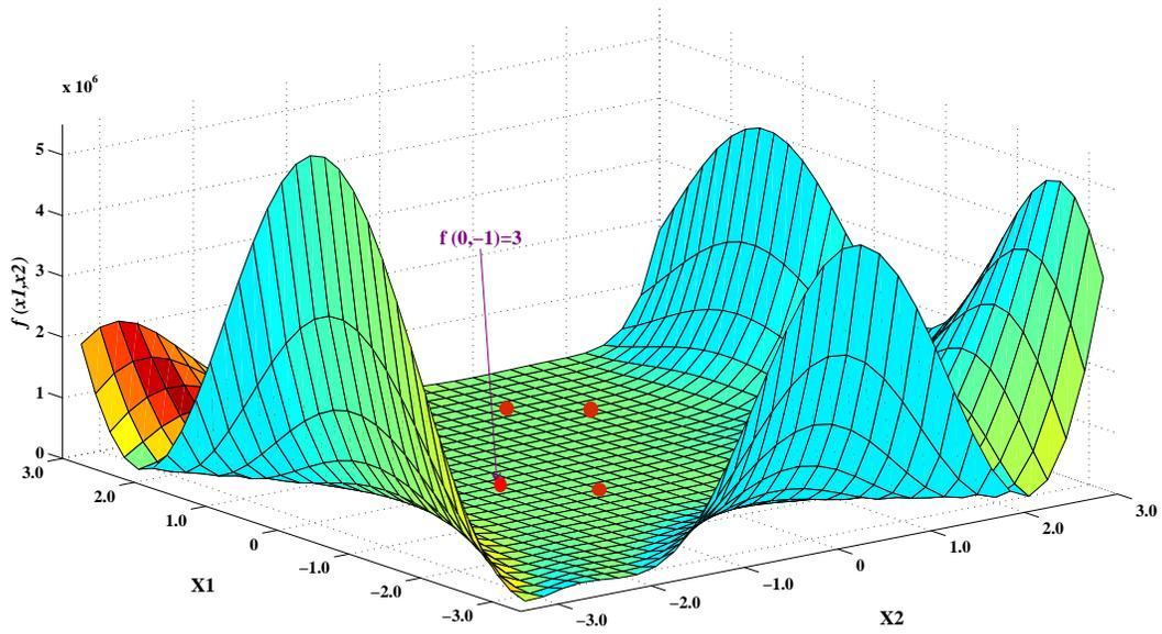
FIG. 2: The potential surface near the global minimum of the GP function (See the text). It is difficult to tell the four minima points visually on a scale of zero to five million, so I marked them by brown circles.  $f(0, -1) = 3$  is the global minimum which was indicated by the arrow.
