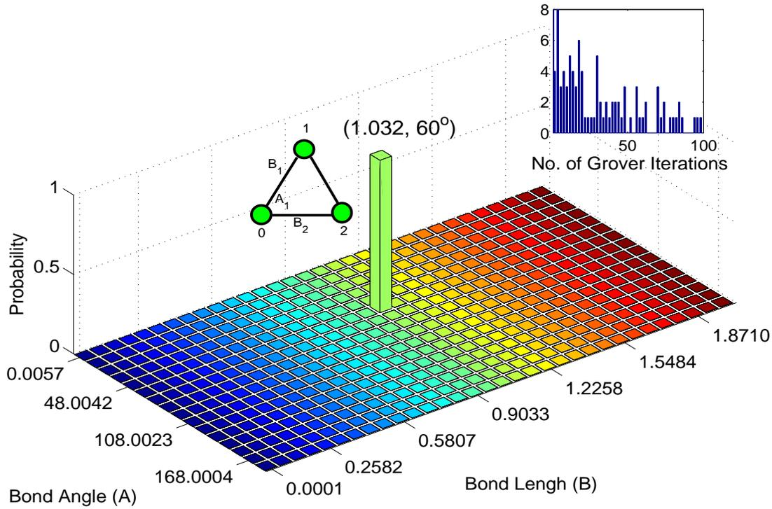
FIG. 4: Final probability distribution of the state function for LJ ( $N=3$ ). The global minimum located at  $B_1 = 1.0323$ ,  $B_2 = 1.0323$  and  $A_1 = 1.0473\text{rad} = 60^\circ$ . The top panel is the distribution of total measure step before reaching the global minimum for 100 search results. The global minimum and corresponding structure are also shown in figure.
