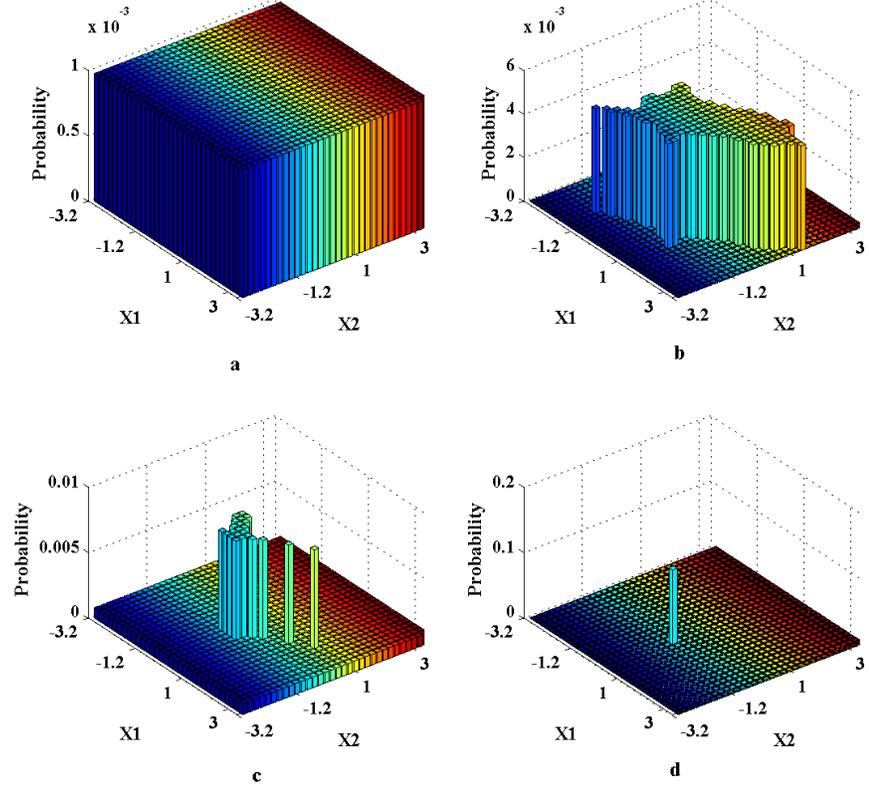
FIG. 3: Probability distribution of the state function before the measurement for the GP function. The panel a is the initial state corresponding to the superposition of all possible states, the panels b, c and d are the distributions of step 5, 10 and 16 respectively.
