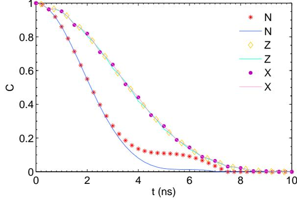
Figure 3: Decay of the entanglement in a radical pair reaction  $[\text{Py-}h_{10}^- \text{DMA-}h_{11}^+]$  under different types of quantum control. (N) without control; (Z) under  $Z$  control, (X) under  $X$  control. The curves are the estimated best lower bounds from the singlet fidelity, the symbols denote the values from numerical simulation. The magnetic field is  $B = 4.5$  mT, and the control time is  $\tau = 0.5$  ns.
