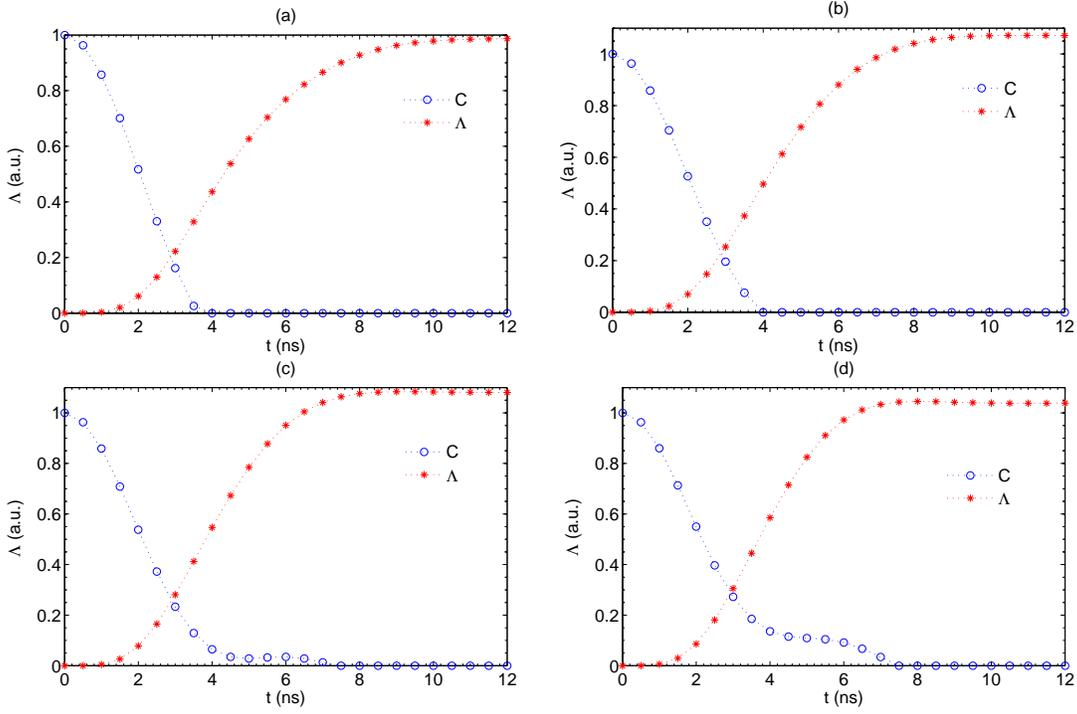
Figure 6: (Color online) Time evolution of the (accumulated) magnetic-field sensitivity  $\Lambda(B, t)$  (rescaled) and the entanglement of the radical pair for (a)  $B = 3\text{mT}$ , (b)  $3.5\text{mT}$ , (c)  $4\text{mT}$ , and (d)  $4.5\text{mT}$  in the radical pair reaction  $[\text{Py}\text{-}h_{10}^-\text{DMA}\text{-}h_{11}^+]$ . The recombination rate constant is  $k = 5.8 \times 10^8 \text{ s}^{-1}$  [1].
