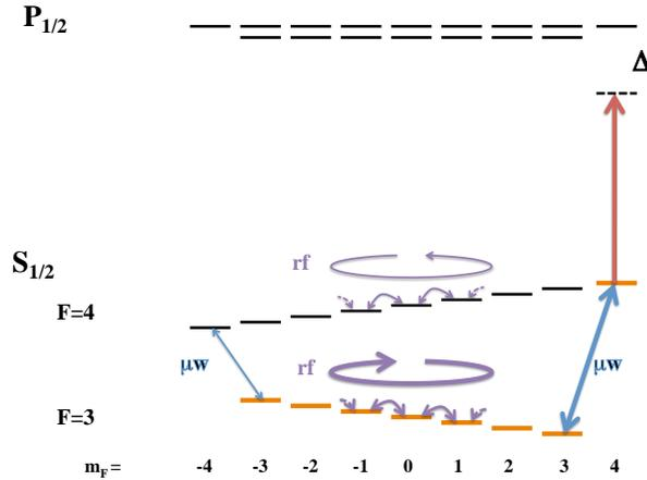
Figure 5.1: The hyperfine structure of  $^{133}\text{Cs}$  in the  $6S_{1/2}$  ground state. Microwaves (blue) and rf magnetic fields (purple) provide controllable dynamics on the 16-dimensional Hilbert space. A detuned laser light shift (red) can be used to create a relative phase between the  $F = 4$  and  $F = 3$  manifolds. By considering controls on the subspace of the orange states we recover a system that satisfies the criteria proposed in chapter 5.1.
