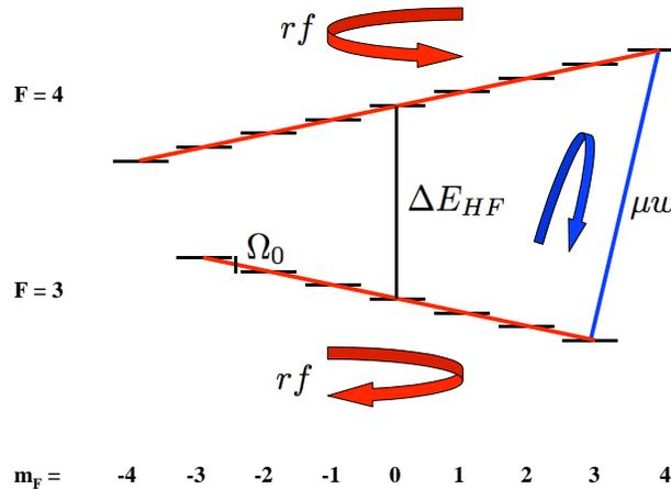
Figure 3.2: The ground state hyperfine manifold of  $^{133}\text{Cs}$ . Rf-magnetic fields (in red) lead to independent rotations in the two manifolds. Microwaves (in blue) are the generators of rotation in a two-dimensional subspace between states in the two manifolds, here the stretched state transition  $|4, 4\rangle \rightarrow |3, 3\rangle$ .
