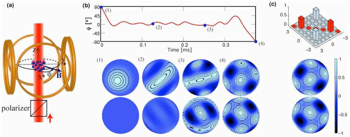
Figure 4.1: Quantum control of a large atomic spin. (a) Schematic of the experiment. (b) Example of a control waveform  $\phi(t)$ . (1-4) Wigner functions at four stages during the control sequence. Both sides of the sphere are shown. The final result is close to the target state  $|\psi_{target}\rangle = (|m_z = 2\rangle + |m_z = -2\rangle)/\sqrt{2}$ . (c) Density matrix (absolute values) and Winger function for  $|\psi_{target}\rangle$
