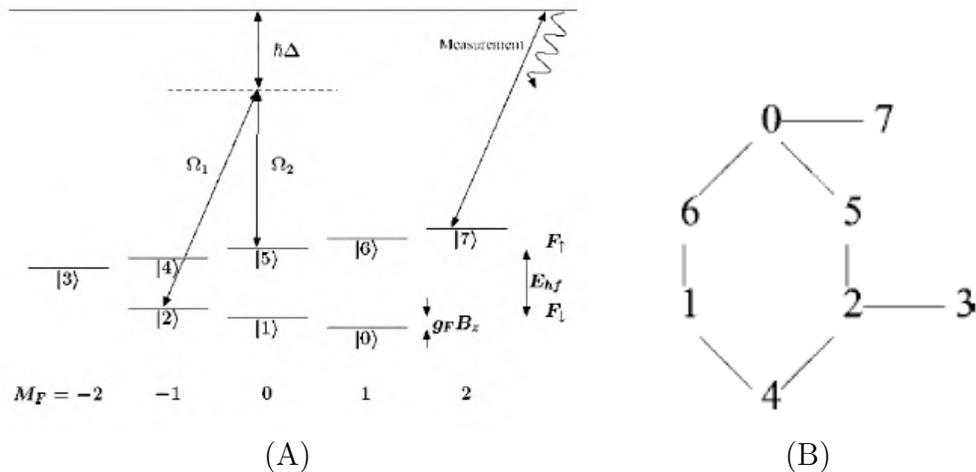
Figure 2.1: In (A) we have an example of a system that allows for the unitary construction technique in this section [15]. The system of interest is the electronic ground state of  $^{87}\text{Rb}$ . The coupling Hamiltonians are realized by two lasers driving Raman transitions. These resonances can only couple hyperfine levels satisfying the selection rules  $\Delta_{m_F} = 0, \pm 1$ , which leads to the connected coupling graph in (B).
