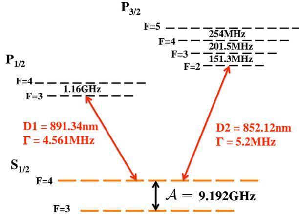
Figure 3.1: The level structure of  $^{133}\text{Cs}$  for the D1 and D2 line. Our control system of interest is the  $S_{1/2}$  ground state, highlighted in orange.
