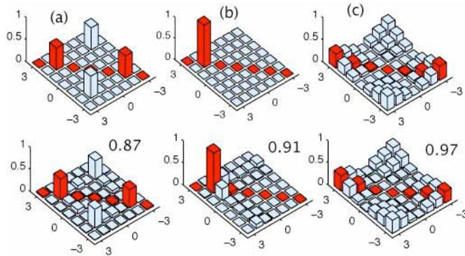
Figure 4.2: Examples of target and measured density matrices (absolute values). The target states are (a)  $(|m_z = 2\rangle + |m_z = -2\rangle)/\sqrt{2}$ , (b)  $|m_x = 2\rangle$ , (c)  $\sum_y m_y |m_y\rangle$ . The experimental yield is indicated for each case.
