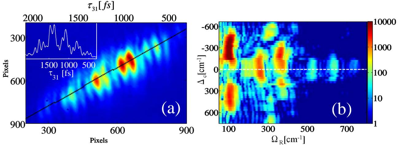
FIG. 3. (Color online) (a) Typical Single Shot FWM image of chloroform with the time resolved FWM signal in the inset. (b) Two dimensional spectrogram of the chloroform Raman FWM signal obtained by phase matching filtering, where the power spectrum of the FWM signal is plotted horizontally against the Raman frequency ( $\Omega_R$ ) and vertically against ( $\Delta_c$ ), the detuning of the PMF from the laser center frequency (log scale).
