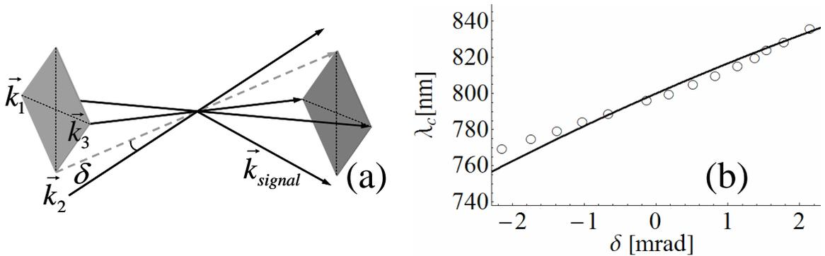
FIG. 2. (a) The 3D-Boxcars configuration, with the Stokes beam deviation angle  $\delta$ . (b) Central frequency of PMF as function of  $\delta$  measured (open circles) and calculated (line).
