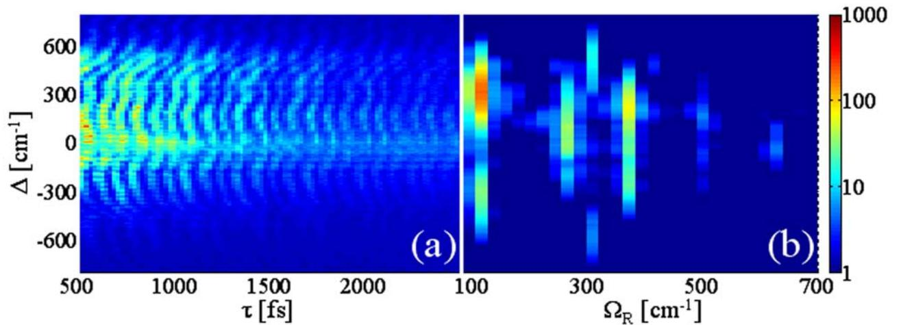
FIG. 1. (Color online) (a) Spectrally and temporally resolved FWM signal from neat chloroform ( $\text{CHCl}_3$ ). (b) Horizontal line by line Fourier Transform of part (a) depicting the power spectrum at each Raman frequency (log scale).
