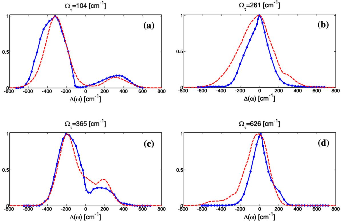
FIG. 4. (Color online) Detuning dependence (normalized) of the Raman contributions and a comparison between the 2D-spectrograms obtained by the Spectrally Resolved Temporal Scanning method (red dashed lines) and by the Single-Shot PMF method (blue lines with solid circles). (a) Depicts section of both spectrograms along  $\Omega_R = 104\text{cm}^{-1}$  (b) along the  $\Omega_R = 261\text{cm}^{-1}$  (c)  $\Omega_R = 365\text{cm}^{-1}$  and (d)  $\Omega_R = 626\text{cm}^{-1}$ .
