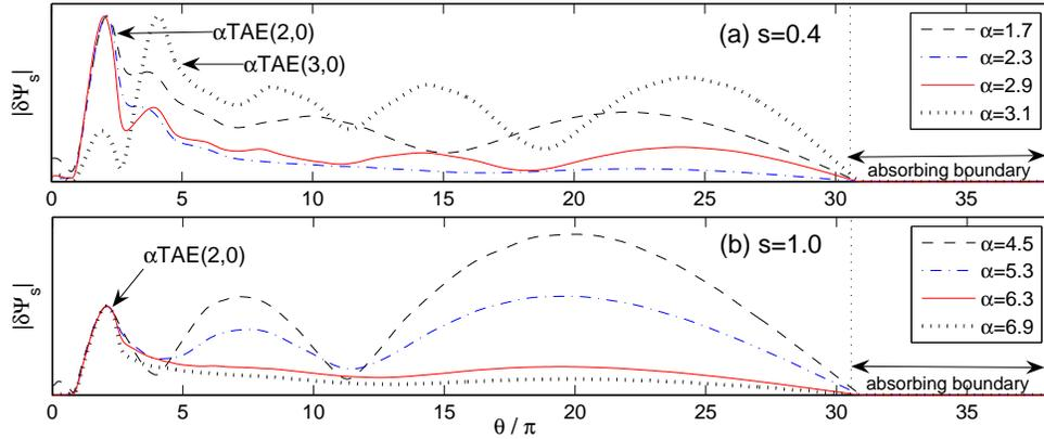
**Figure 3.** Mode structures  $|\delta\Psi_s(\theta)|$  of ITG-driven  $\alpha$ TAEs for several values of  $\alpha$ . (a):  $s = 0.4$ , modes in regions (IVa) and (V) of figure 1. (b):  $s = 1.0$ , modes in region (IVa) of figure 2.
