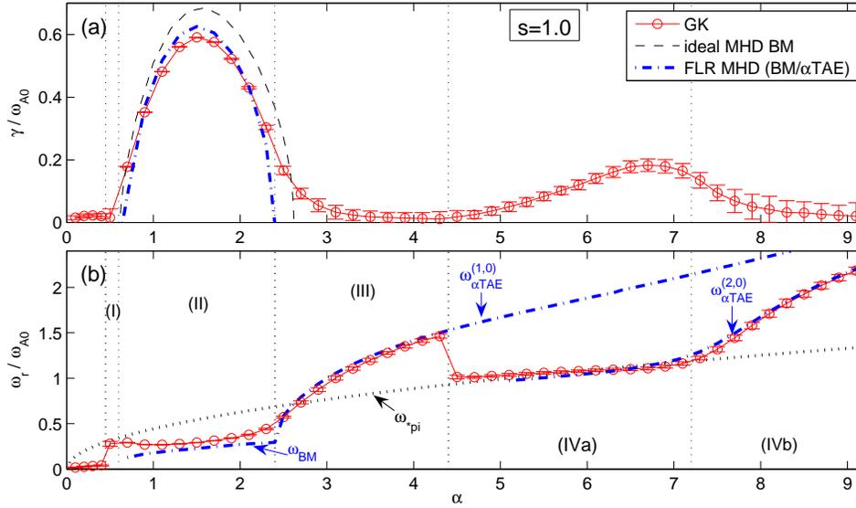
**Figure 2.** High shear case,  $s = 1.0$ .  $\alpha$ -dependence of (a) the growth rate  $\gamma$  and (b) the frequency  $\omega_r$ . Arranged as figure 1. Here, the thermal transit frequency,  $\omega_{ti}$ , is about a factor 4 smaller than  $\omega_{*pi}$ .
