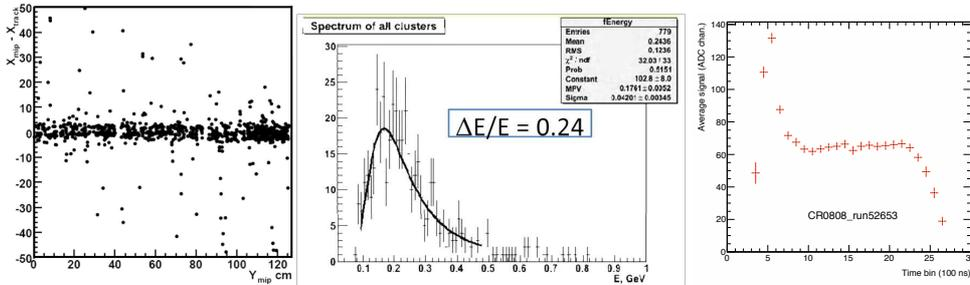
Figure 6: Left panel: HMP-TPC track matching. Centre panel: PHO energy resolution for cosmic muons. Right panel: First TRD signals.
