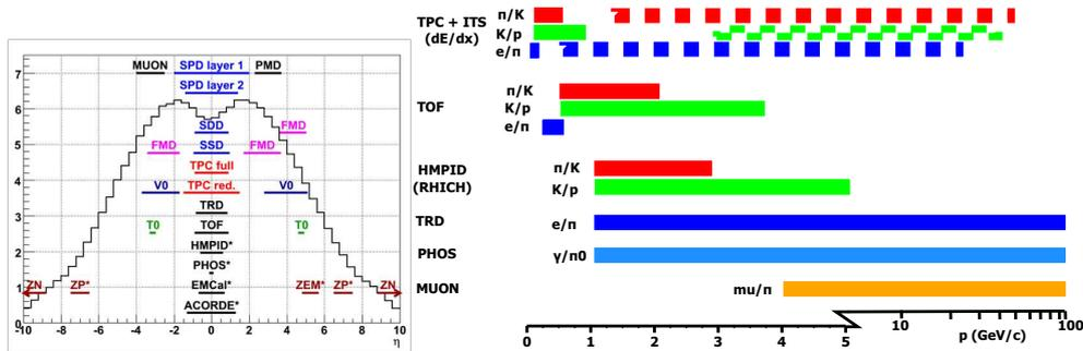
Figure 1: ALICE Pseudo rapidity coverage of the ALICE detectors (left panel), and the particle identification capabilities of the detectors (right panel).
