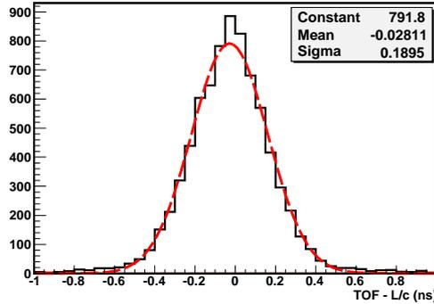
Figure 5: Time of flight distribution measured using cosmic muons. The time resolution of a single module is found by dividing the width of the distribution by  $\sqrt{2}$ , i.e. 130 ps.
