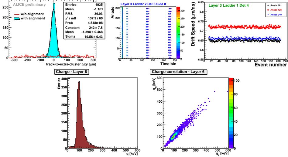
Figure 3: Calibration and alignment results for the inner tracking system. Upper left: track to track distance before and after alignment. Upper middle panel: drift speed map of a silicon drift detector. Upper right panel: Drift speed as a function of time for a silicon drift detector. Lower left panel: measured energy loss in a silicon strip detector after calibration. Lower right panel: Measured charge correlation between the two sides of a silicon strip detector
