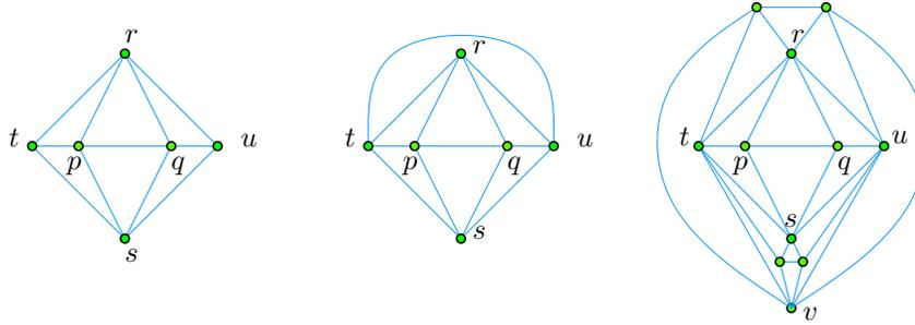
**Fig. 21.** Left: vertex labeling for Lemma 24; right and center: the two indecomposable graphs for the lemma, the octahedral graph  $\Delta_6$  and an 11-vertex graph  $\Delta_{11}$  formed by adding two vertices inside each face of the complete bipartite graph  $K_{2,3}$ .
