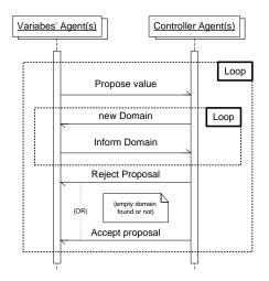
Figure 7. Implementation of interaction during value proposing stage
