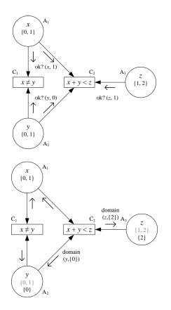
Figure 4. Illustration of value proposing and validating stage of CACS.
