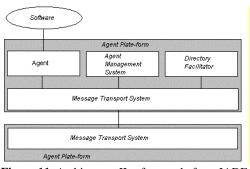
Figure 11. Architecture II software platform JADE
