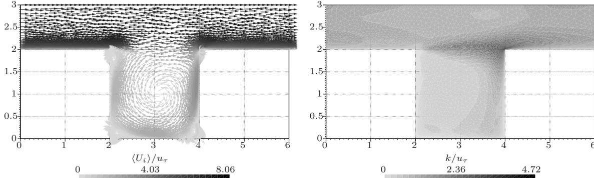
Fig. 18. Mean velocity vectors (left) and contourlines of turbulent kinetic energy (right) of a fully developed turbulent street canyon at  $Re_\tau \approx 600$  based on the friction velocity and the free-stream height.
