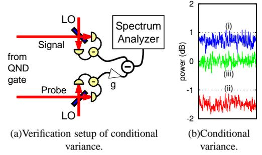
FIG. 8: (Color online) Verification setup and experimental results of conditional variance of the signal  $x$ -quadrature when the probe  $x$ -quadrature is measured. Here both the signal and probe are measured via homodyne-detectors, their outcomes are electrically subtracted in the optimal gain  $g = 0.56$  and measured by spectrum analyzer. The signal  $x$ -quadrature variance [trace (i)] is reduced by measuring  $x$ -quadrature of probe (ii), and suppressed below the shot-noise limit (iii).
