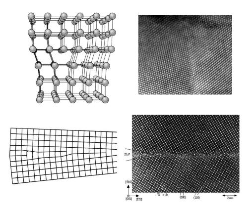
Figure 1: Edge dislocation and small angle grain boundary. The pictures on the left are from [Ki] with kind permission of the publisher. The pictures on the right were taken with a TEM; references:
