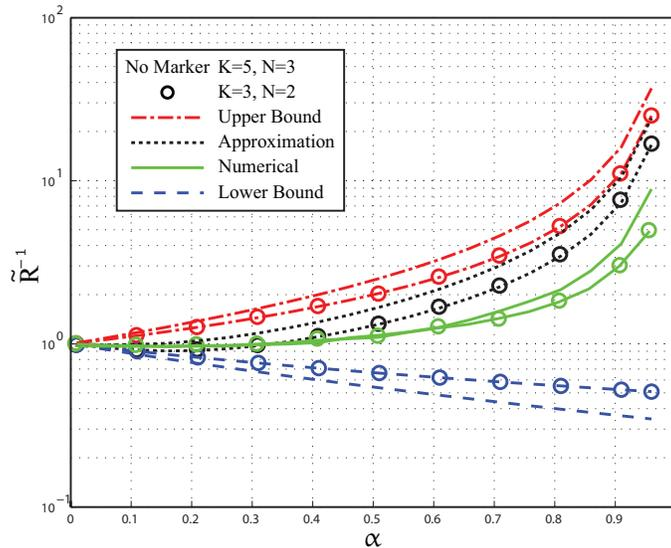
Fig. 2. Comparison of the numerical values of  $\tilde{R}_i^{-1}$  with the proposed approximation and the bounds in Section III in two MIMO IA networks, a 3-user  $2 \times 2$  and a 5-user  $3 \times 3$ , for varying antenna correlation values. As expected, the approximation is closer to the true value compared to the bounds. The proposed approximation is within 10% of the true value for  $\alpha < 0.3$ .
