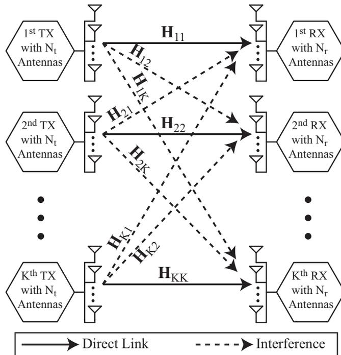
Fig. 1. A  $K$ -user MIMO interference channel where transmitters and receivers have  $N_t$  and  $N_r$  antennas respectively.
