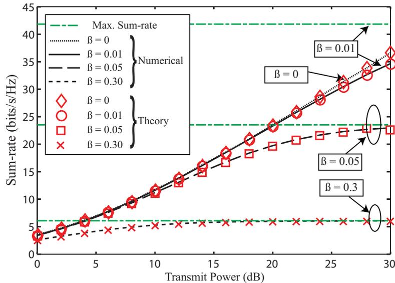
Fig. 4. Theoretical predictions and numerical results for the sum rate of a 4-user  $3 \times 3$  constant channel MIMO IA ( $\alpha = 0$ ) for 4 values of  $\beta$  versus  $\gamma_o$ . As can be seen, numerical simulations closely follow the analytical curves and the theoretical maximum sum rates correctly predict the upper bounds for the given  $\beta$ .
