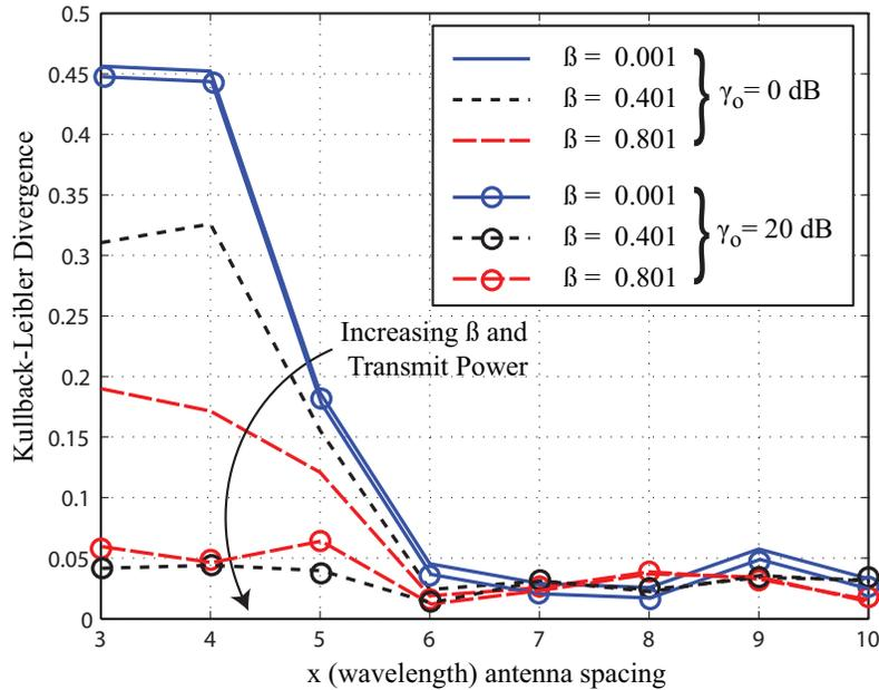
Fig. 3. Kullback-Leibler divergence between the theoretical distribution of the per-stream received SINR given by (29) and the true distribution found through numerical simulation as a function of  $\alpha$  for varying  $\beta$  and  $\gamma_o$ . As can be seen, the accuracy of (29) increases with increasing  $\beta$  and transmit power.
