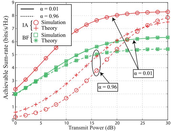
Fig. 5. Achievable sum rate of 3-user  $2 \times 2$  IA MIMO network and a  $2 \times 2$  MIMO beamforming link as a function of  $\gamma_0$  for varying  $\alpha$  and a fixed  $\beta = 0.19$ . The accuracy of (29) increases with increasing  $\gamma_0$  and decreases with increasing  $\alpha$ . As can be seen, beamforming can outperform IA for a wide range of parameters. Moreover, Lemma 5 can be used to accurately predict the beamforming performance.
