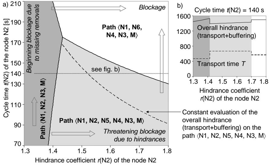
**Fig. 14** a) Path finding as a function of cycle time  $t(N2)$  and hindrance coefficient  $r(N2)$  of node N2. The dashed line corresponds to the isocline of constant hindrance. b) Overall hindrance and transport time  $T$  along the isocline  $t(N2) = 140$  s as a function of the hindrance coefficient  $r(N2)$ . One can see that the overall hindrance may drop, while the transport time  $T$  increases.
