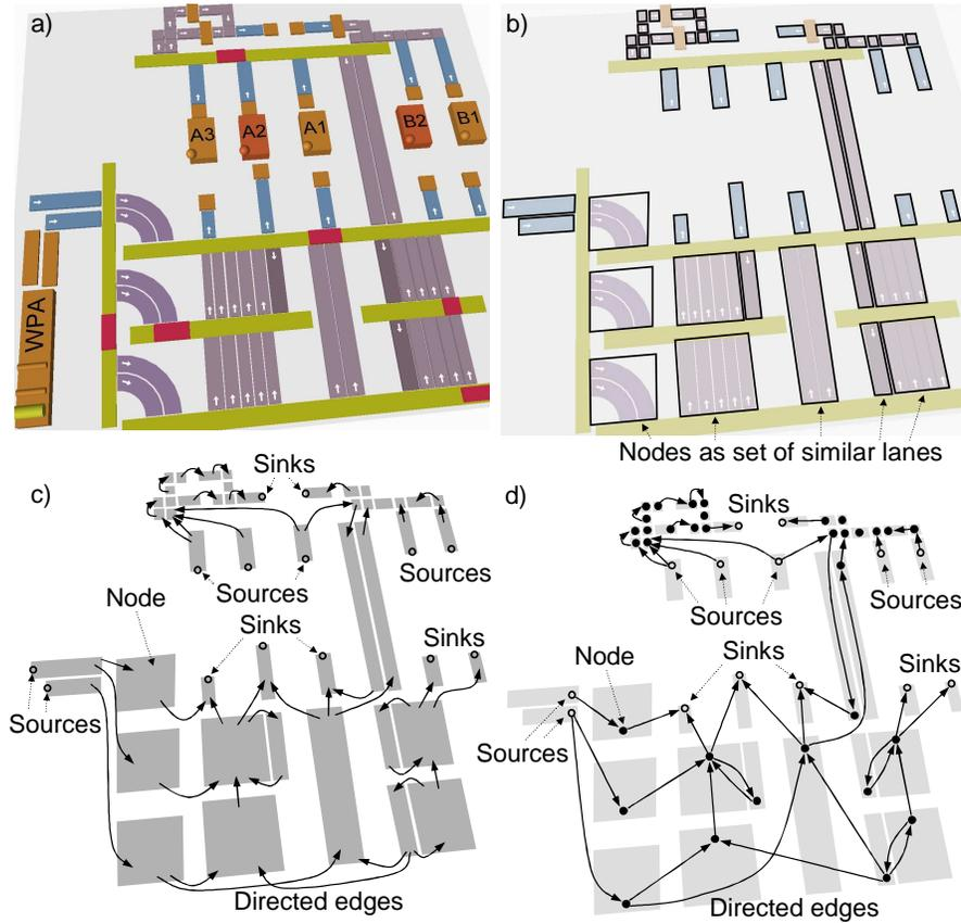
**Fig. 9** Different steps in the abstraction of a factory layout. a) Example of a plant layout. b) Logical representation of the buffer system as a set of nodes of a mathematical graph. c) Representation of the transfer cars and the dispatch machines as directed edges of the graph (only a subset of edges is represented). d) Resulting mathematical graph representing the factory layout.
