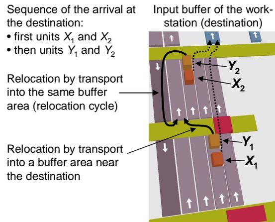
**Fig. 2** To meet the scheduled arrival sequence, relocations may be required to process or finish units in the right order: In this illustration, the units  $Y_1$  and  $Y_2$  have to relocate, as they obstruct the units  $X_1$  and  $X_2$ .
