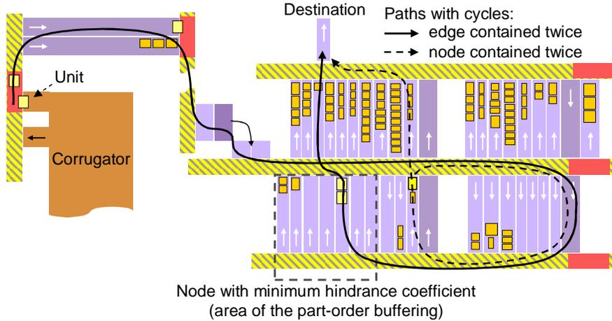
**Fig. 8** Illustration of two paths containing the same edge twice (solid line) or the same node twice (dashed line). Cycles are generated by selecting a hindrance-minimal buffer area (i.e. the node with smallest hindrance coefficient).
