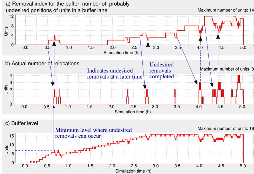
**Fig. 5** Comparison of the relocation cycles with the removal index and number of units for a buffer area with 2 lanes and 8 positions each. a) Removal index. b) Amount of transfer lane necessary for the relocation cycles. The causal influences are represented by arrows. c) Buffer level.
