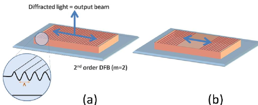
**Figure 7** (a) DFB structure directly engraved onto a polymeric film. If  $\Lambda = \lambda/n_{eff}$  ( $2^{nd}$  order grating,  $m=2$ ) then a diffracted beam (first diffraction order) is emitted in the direction perpendicular to the film plane (b) DBR structure with no corrugation between two Bragg mirrors.
