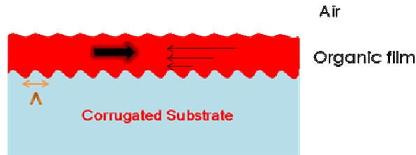
**Figure 6** Possible structure of a DFB laser where the organic film is deposited on a pre-corrugated substrate with a modulation period equal to  $\Lambda = m\lambda/2n_{\text{eff}}$ . The light propagating from the left is scattered by the corrugation, and the diffracted waves interfere constructively in the opposite direction, creating a counterpropagating wave.
