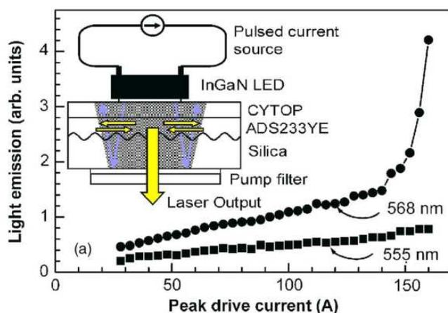
**Figure 12** : Performance of the LED-pumped organic laser proposed by the Ifor Samuel's group. The LED was manufactured by Philips (Luxeon) and driven with short current pulse to reach lasing threshold (details in ref [153]). Inset : scheme of the device : the resonator is a 2<sup>nd</sup> order DFB grating. Courtesy of Ifor Samuel. Reprinted with permission from [28]. Copyright 2011, American Institute of Physics.
