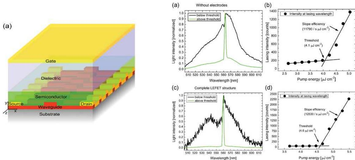
**figure 11** : Left : a Light-emitting field-effect transistor (LEFET) structure incorporating a DFB grating for lasing applications. Right : Spectra and laser curves of the structure without (on top) and with electrodes (bottom). Courtesy of Henning Sirringhaus. Reprinted with permission from [148]. Copyright 2011 John Wiley and Sons.
