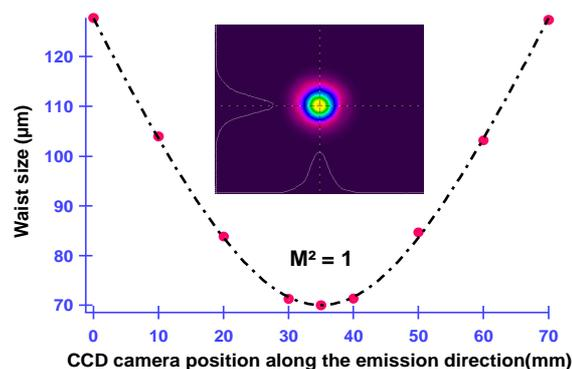
**Figure 15** : CCD image of the beam profile and  $M^2$  measurement of a Vertical External Cavity Surface-emitting Organic Laser, from ref [121] ( $M^2$  is defined as the ratio of the divergence to the theoretical diffraction-limited divergence.) Reprinted with permission from [172]. Copyright 2011, Optical Society of America.
