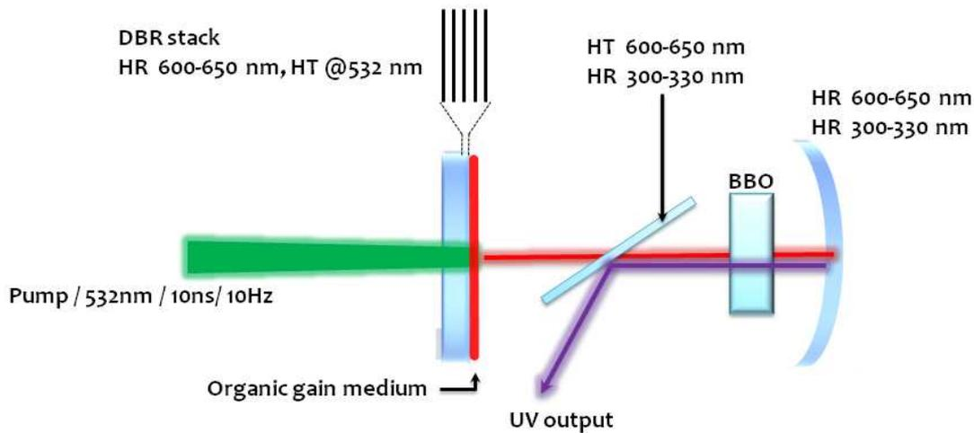
**Figure 13** : Tunable UV organic laser based on a modified VECSOL[30]: a nonlinear crystal is inserted inside the resonator to benefit from the high peak power. A dichroic plate in the cavity allows for the extraction of the UV beam and avoids any accelerated degradation due to the interaction between UV photons and the organic layer. Reprinted with permission from[30] . Copyright 2011, American Institute of Physics.
