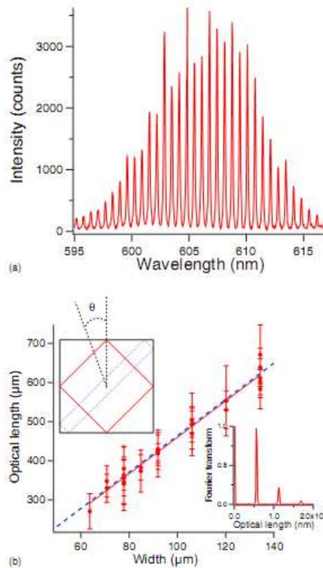
**Figure 9** : optical spectrum obtained from a square-shaped PMMA:DCM microlaser (square width  $W=150 \mu\text{m}$ ), from ref.[119] (b) : a Fourier transform (inset) of the spectrum allows inferring directly the length of the periodic orbit, which as expected is found to vary linearly with the square dimension  $W$ . Reprinted figure with permission from [119]. Copyright 2011 by the American Physical Society.
