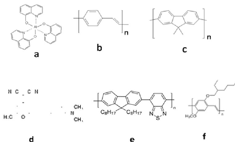
**Figure 2 :** Chemical structure of some typical organic media used in organic lasers : (a) aluminium tris(quinolate) or Alq<sub>3</sub>- (b) generic polyphenylene vinylene or PPV (c) generic polyfluorene (d) DCM (4-(Dicyanomethylene)-2-methyl-6-(4-dimethylaminostyryl)-4H-pyran (e) F8BT [poly(9,9'-dioctylfluorene-co-benzothiadiazole)] (f) MEH-PPV [poly(2-méthoxy-5-(2-éthyl-hexyloxy)-1,4-phenylene-vinylene)]
