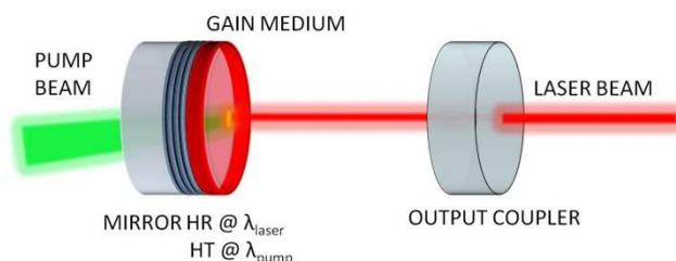
**Figure 10** : a Vertical External Cavity Surface-emitting Organic Laser (VECSOL)[121] . The left mirror is transparent for the pump wavelength and highly reflective for the laser radiation. The output coupler radius-of-curvature and reflectivity are optimized to yield the highest output energy in a single transverse mode.
