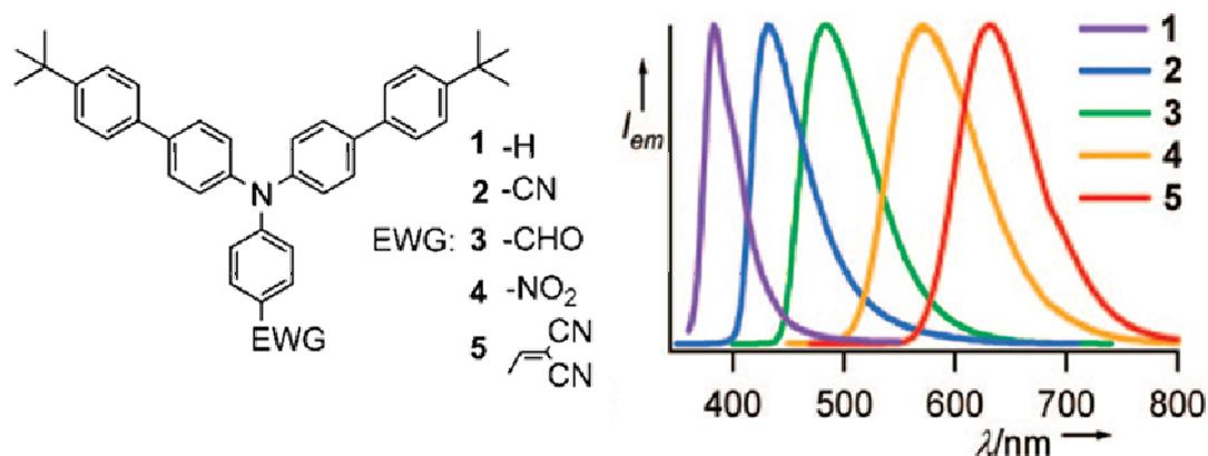
**Figure 5:** Illustration of chemical tuning by substitution of different Electron-Withdrawing Groups (EWG) on a triphenylamino moiety. Right : fluorescence spectra of 100-nm-thick evaporated neat films. Courtesy of E. Ishow. Reprinted with permission from [45]. Copyright 2011 American Chemical Society.
