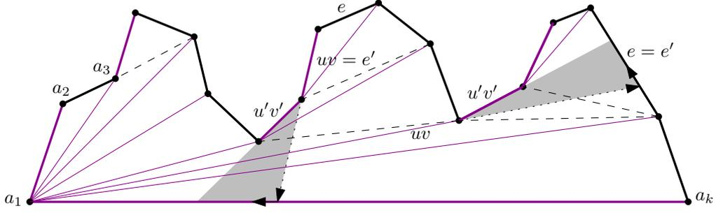
Figure 2: The shortest path tree SPT from  $a_1$  to all other vertices (in purple). Additional triangulation edges generated in our algorithm are dashed. The figure illustrates a forward step (right shaded area) and a backward step (middle area).
