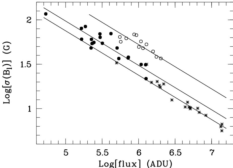
Fig. 10.— The uncertainty of the longitudinal magnetic field as measured with *dimaPol* as a function of source flux. Data for the Sun and two magnetic null standard stars are shown: stars - scattered solar light, filled points -  $\iota$  Peg, open points -  $\gamma$  Peg. The solid lines show the  $\sqrt{\text{flux}}$  fit for each source.
