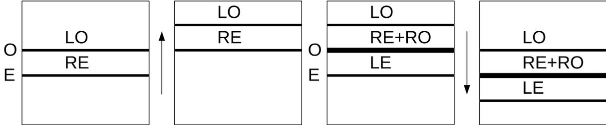
Fig. 6.— A schematic representation of one switch cycle of *dimaPol*. From left to right: expose, move the accumulated charge up, switch the FLC wave plate and expose again, move the charge back down and switch the wave plate in preparation for the start of the next switch cycle. As a result, three spectra form on the CCD (see text).
