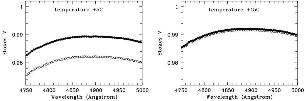
Fig. 5.— Depolarization due to crosstalk between the two channels of *dimaPol* (open circles). 100% input circular polarization is assumed (Stokes V equal to 1). The crosstalk can be significantly reduced by rotating the FLC plate by  $2^\circ$  (filled circles).
