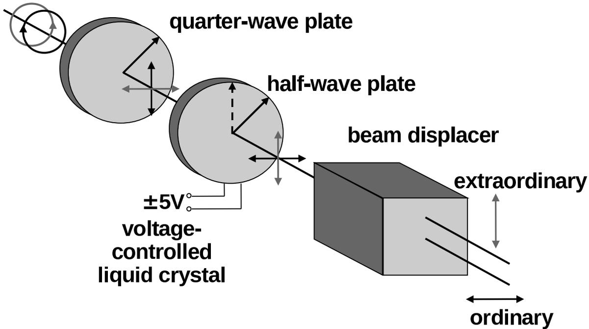
Fig. 1.— A sketch of the optical layout of the polarimetric module.
