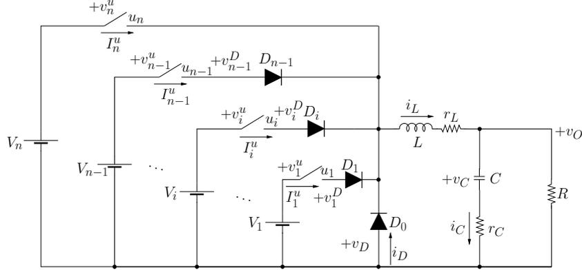
Figure 8: Multi-input Buck DC-DC Converter.
