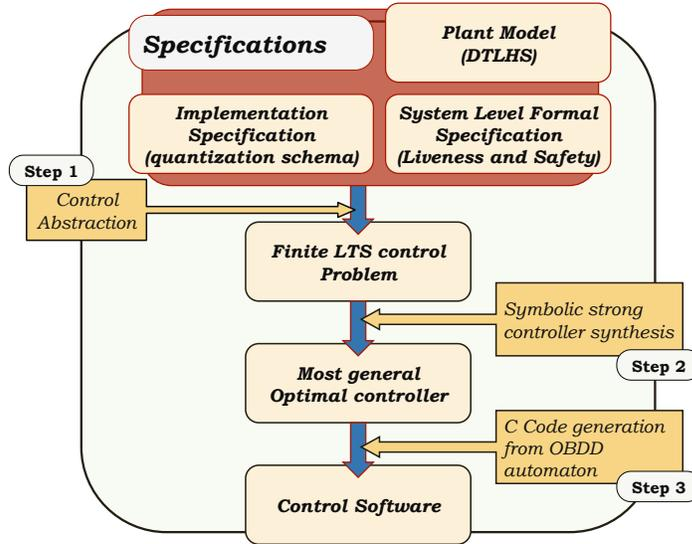
Figure 1: Control Software Synthesis Flow.
