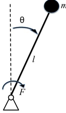
Figure 7: Inverted Pendulum with Stationary Pivot Point.
