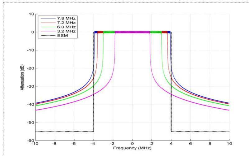
Figure 3: OFDM+CP vs. ESM, original picture [5]
