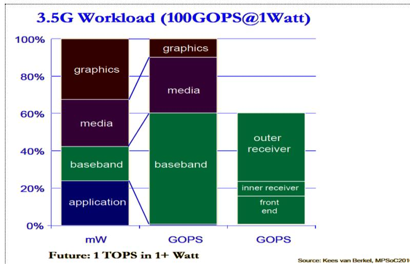
Figure 4: Workload of current mobiles (outer receiver consists of channel decoder and de-interleaver)
