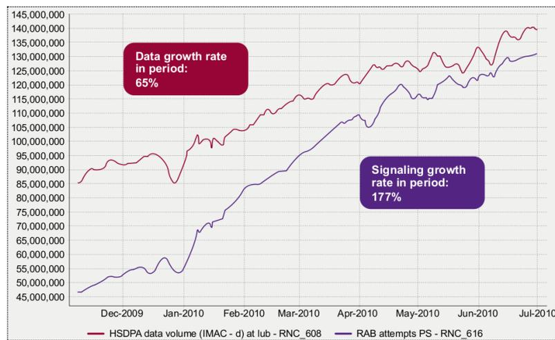
Figure 2: Comparisons of data and signalling traffic [2]
