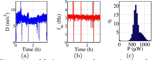
**Figure 6:** Motion energy characterization for a 3 hour run: (a) the absolute deviation of acceleration,  $D$ , and (b) dominant motion frequency,  $f_m$ , as functions of time, and (c) the distribution of the corresponding power harvested,  $P(t)$ .
