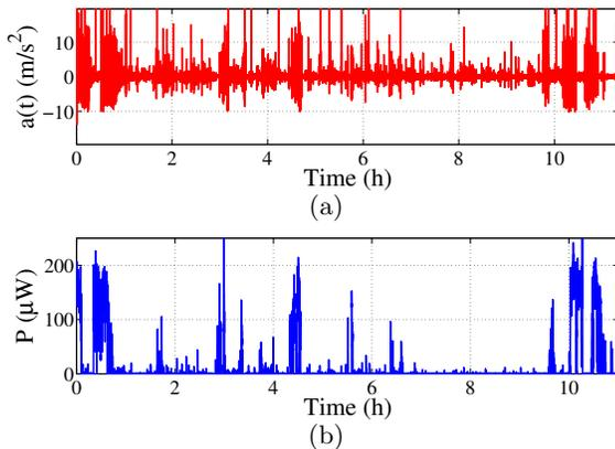
**Figure 7: Kinetic energy for normal daily human routine: (a) acceleration,  $a(t)$ , recorded over 11 hours for participant M5, and (b) the power harvested,  $P(t)$ .**
