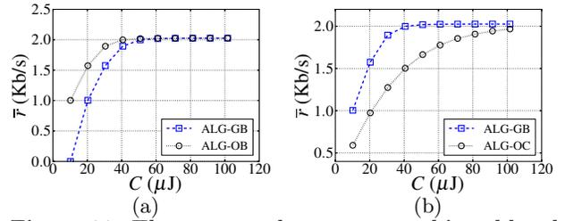
**Figure 11:** The average data rate,  $\bar{r}$ , achieved by the algorithms using energy traces for participant  $M1$ , for (a) the battery model, for  $B_K = B_0 = 10 \cdot s_{\text{min}}$ , and (b) the battery and capacitor models.
