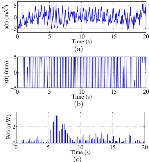
**Figure 3: Demonstration of obtaining the power generated by a harvester,  $P(t)$ , from the recorded acceleration,  $a(t)$ :** (a)  $a(t)$  recorded by a person walking, (b) the corresponding harvester proof mass displacement,  $z(t)$ , and (c) the resulting  $P(t)$  for harvester H1 ( $k = 0.17$ ,  $b = 0.0055$ ).
