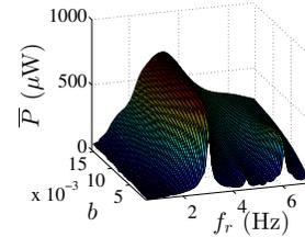
**Figure 4: The average power generated by a harvester,  $\bar{P}$ , from the same motion (human running) for different combinations of harvester resonant frequencies,  $f_r$ , and damping factors,  $b$ .**
