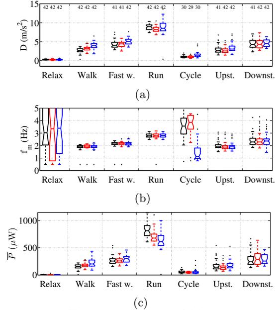
**Figure 5: Characterization of kinetic energy for common human activities, based on a 40-participant study: (a) average absolute deviation of acceleration,  $D$ , (b) dominant motion frequency,  $f_m$ , and (c) power harvested by an optimized harvester,  $\bar{P}$ .**
