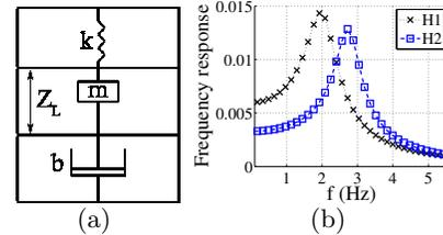
**Figure 1: (a) A second-order mass-spring system model of a harvester with proof mass  $m$ , proof mass displacement limit  $Z_L$ , spring constant  $k$ , and damping factor  $b$ , and (b) the frequency response magnitude for harvesters  $H1$  and  $H2$ .**
