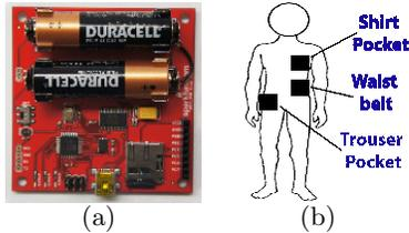
**Figure 2: Acceleration measurement unit and placements:** (a) our sensing unit based on a SparkFun ADXL345 board, and (b) the sensing unit placements in a multi-participant human motion characterization study [40].
