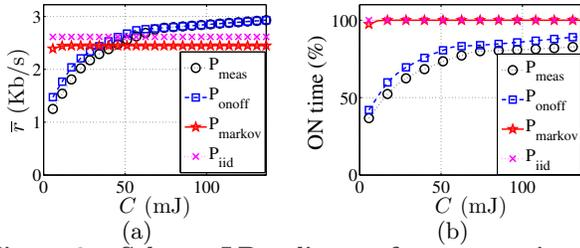
**Figure 9: Scheme-LB policy performance using energy traces ( $P_{\text{meas}}$ ) for participant M1 and using the corresponding ON/OFF ( $P_{\text{onoff}}$ ), Markov ( $P_{\text{markov}}$ ), and i.i.d. ( $P_{\text{iid}}$ ) processes: (a) average data rates,  $\bar{r}$ , and (b) node ON times.**
