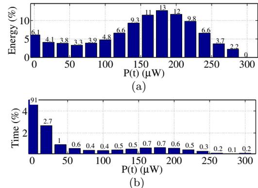
**Figure 8: Motion energy harvesting process variability for participant M1: (a) the percentage of the total energy harvested at different power levels  $P(t)$ , and (b) the percentage of time the power is harvested at the different  $P(t)$  (notice that for  $0 \leq P(t) \leq 15$ , the value is 91%).**
