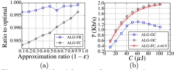
**Figure 10:** Algorithm performance using energy traces for participant  $M1$ , for: (a) battery and capacitor models, performance ratio between ALG-FC (ALG-FB) and ALG-OC (ALG-OB), and (b) the capacitor model, average data rate,  $\bar{r}$ , achieved by different algorithms.
