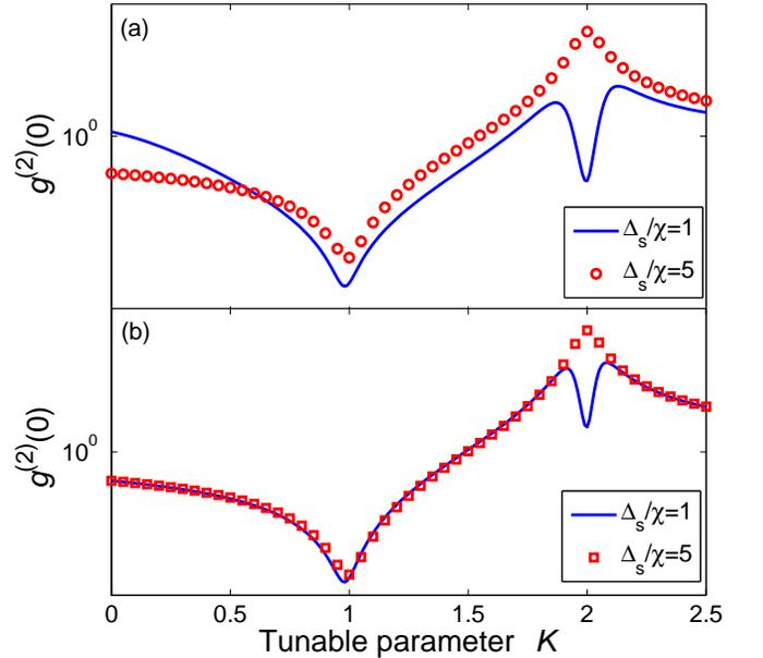
FIG. 6: (a)  $g^{(2)}(0)$  for the controlled TLR and (b)  $g^{(2)}(0)$  for the controller versus the parameter  $K = \Delta/\chi + 1$ . The red dotted curve and the blue curve correspond to different detuning frequencies  $\Delta_s = 50$  MHz and  $\Delta_s = 10$  MHz. The other system parameters are:  $\chi = 10$  MHz,  $\gamma/2\pi = 2$  MHz,  $\gamma_f/2\pi = 2.5$  MHz,  $\kappa = 1$  MHz, and  $\varepsilon = 0.1\kappa$ .
