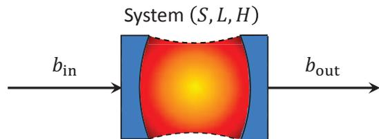
FIG. 1: (Color online) Schematic diagram of the quantum input-output system with the input field  $b_{\text{in}}$  and the output field  $b_{\text{out}}$ . Here,  $S$ ,  $L$ ,  $H$  are, respectively, the scattering matrices, the Lindblad operator, and the Hamiltonian of the input-output system.
