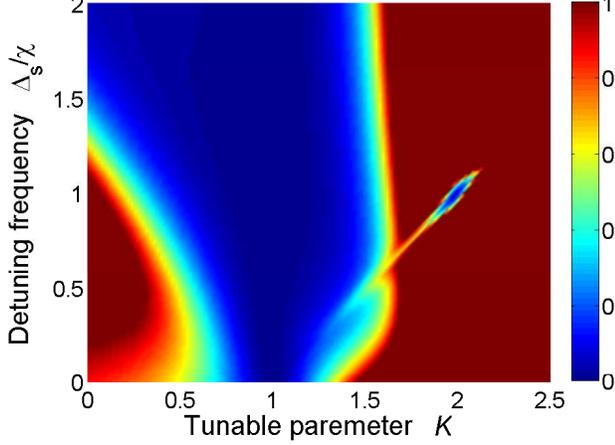
FIG. 7: (Color online). Second-order correlation function versus  $K$  and  $\Delta_s$ , with  $\chi = 10$  MHz,  $\gamma/2\pi = 2$  MHz,  $\gamma_f/2\pi = 2.5$  MHz,  $\kappa = 1$  MHz and  $\varepsilon = 0.1\kappa$ . Note that  $g^{(2)}(0) < 1$  occurs when  $\Delta_s - (K - 1) = 0$ , namely,  $\omega = \omega_s$  and  $K = 1$  with any  $\Delta_s$ .
