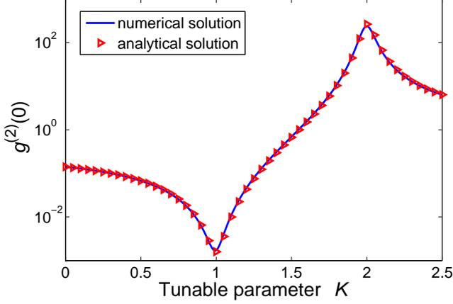
FIG. 5: (Color online). The numerical and analytical solutions for the second-order correlation function  $g^{(2)}(0)$  in Eq. (25) versus the tunable parameter  $K$ . The system parameters for this simulation are:  $\chi = 10$  MHz,  $\Delta_s = 50$  MHz,  $\gamma/2\pi = 2$  MHz,  $\gamma_f/2\pi = 2.5$  MHz,  $\kappa = 1$  MHz, and  $\varepsilon = 0.1\kappa$ .
