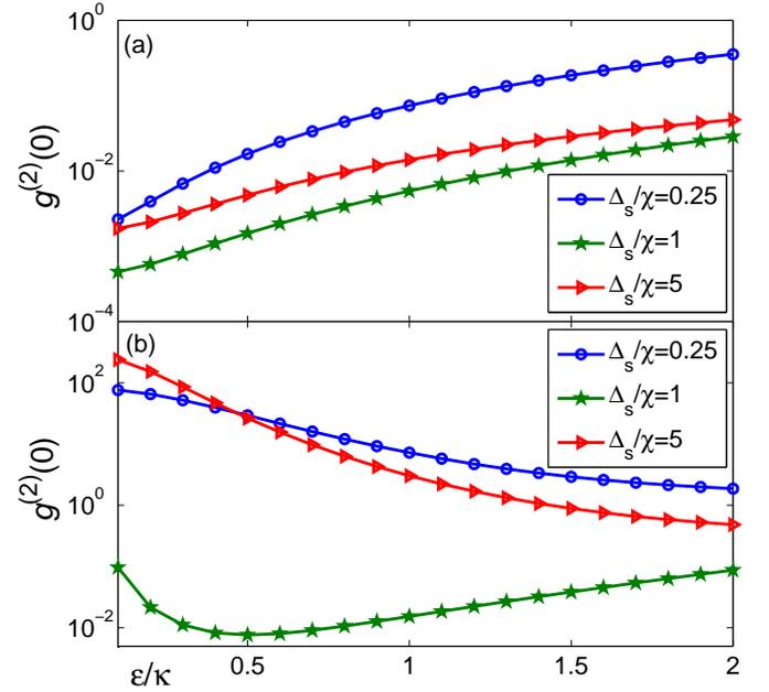
FIG. 8: (Color online). Second-order correlation function versus the normalized driving strength  $\varepsilon/\kappa$ , for different values of the detuning frequency  $\Delta_s$ . Here the system parameters are:  $\chi = 10$  MHz,  $\gamma/2\pi = 2$  MHz,  $\gamma_f/2\pi = 2.5$  MHz, and  $\kappa = 1$  MHz. (a) for  $K = 1$  and (b) for  $K = 2$ .
