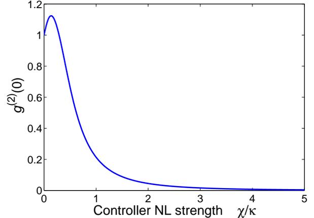
FIG. 9: (Color online). Second-order correlation function versus the nonlinear strength  $\chi$  of the controller, where the parameters of the system are:  $K = 1$ ,  $\gamma/2\pi = 2$  MHz,  $\gamma_f/2\pi = 2.5$  MHz,  $\kappa = 1$  MHz and  $\varepsilon = 0.1\kappa$ .
