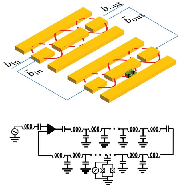
FIG. 3: (Color online) Schematic diagram of the coherent feedback network using superconducting quantum circuits. The controlled system is a TLR which can be considered as a linear cavity. The controller in the feedback loop is another TLR coupled with a dc-SQUID-based superconducting charge qubit which acts as a nonlinear component.
