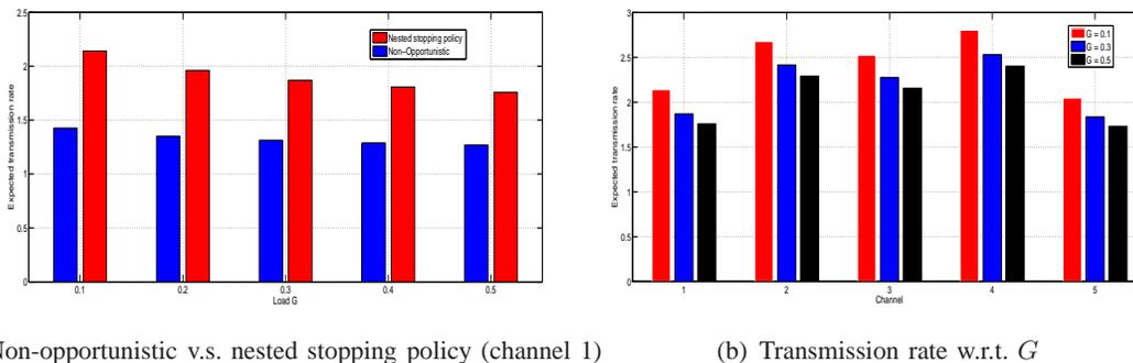
Fig. 4. Performance comparison under an AWGN wireless link model
