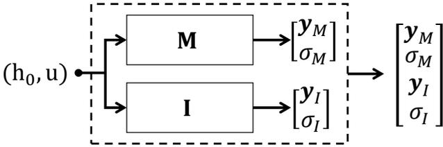
Figure 2: Parallel interconnection of Model and Implementation.
