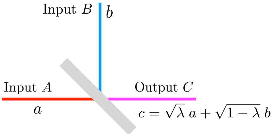
FIG. 1. Graphical representation of the coherent mixing of the two inputs  $A$  and  $B$ . For the quantum mechanical analogue the two input signals correspond to electromagnetic modes which are coherently mixed at a beam-splitter of transmissivity  $\lambda$ . The entropy of the output signal is lower bounded by a function of the input entropies via the quantum entropy power inequality defined in Eq. (5).
