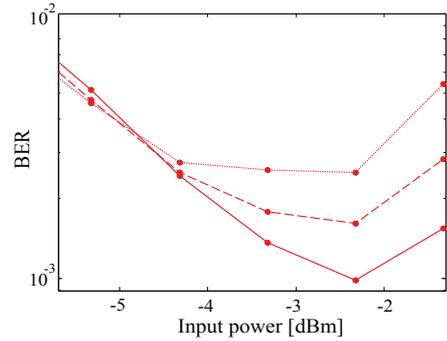
**Fig. 3:** The BER as a function of input power in a 6000 km Raman amplified system. Dotted – without mitigating inter-channel NLIN, solid – mitigation of  $\mathbf{H}_0^{(n)}$ , dashed – mitigation of only the diagonal elements in  $\mathbf{H}_0^{(n)}$ . At very low powers mitigation spoils performance as a result of poor estimation caused by ASE.
