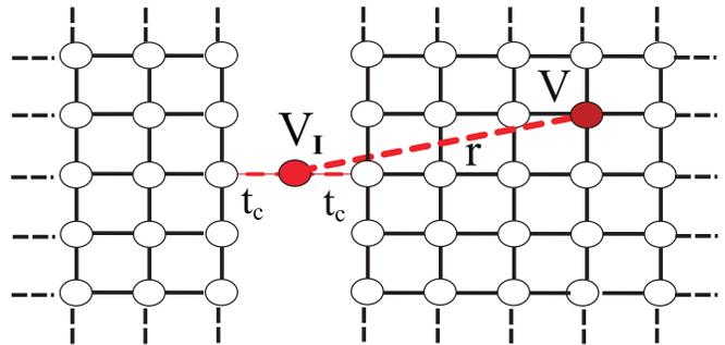
FIG. 3: (Color online) RCM model for the SGM of a quantum contact: Two semi-infinite square lattices are contacted via a single site  $\mathbf{I}$  of coordinates  $(0, 0)$ , potential  $-4t + V_I$  and coupling term  $t_c$ . Taking a potential  $-4t + V$  at another single site  $\mathbf{T}$  of coordinates  $(x, y)$  gives rise to an electron interferometer of size  $r = \sqrt{x^2 + y^2}$ .
