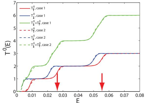
FIG. 16: (Color online) Lattice model (see Fig. 2) of a QPC without tip ( $V = 0$ ) with  $L_y = 20$ ,  $L_x = 16$  and  $k = 2$ : Transmission  $T_{\sigma}^0$  of an electron of spin  $\sigma$  and total transmission  $T^0 = \sum_{\sigma} T_{\sigma}^0$  as a function of  $E$  when a parallel magnetic field  $h = 0.0025$  is applied everywhere (case 1) and only upon the contact region  $-L_x \leq x \leq L_x$  (case 2). The arrows give energies around which beating effects can be seen.
