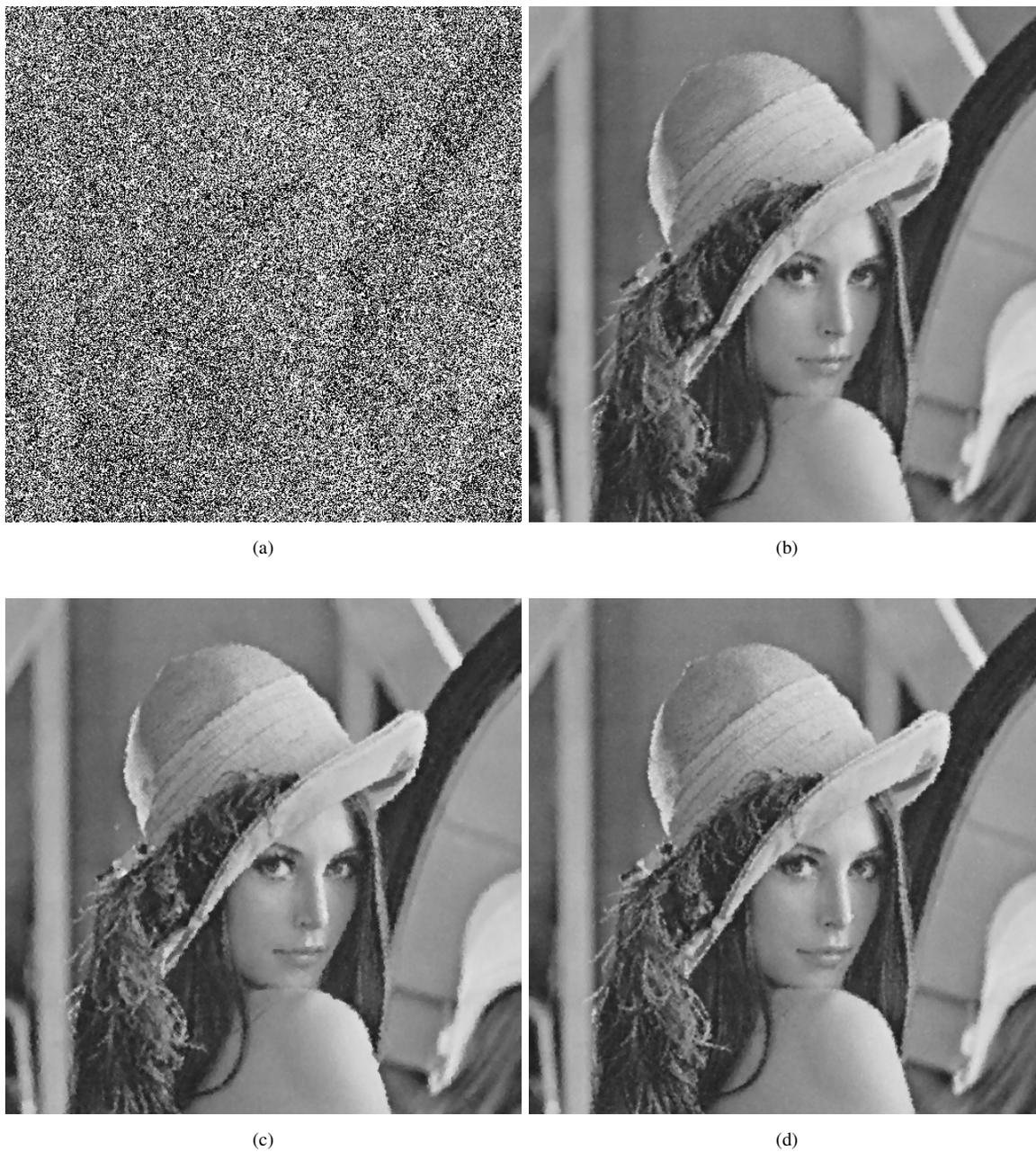
Fig. 3: Restored images using different filters for image *Lena* corrupted by 80% SPN. (a) Corrupted image (6.42 dB), (b) EPA [5] (29.11 dB), (c) SAWM [7] (28.87 dB), (d) EWA [Proposed] (29.61 dB)
